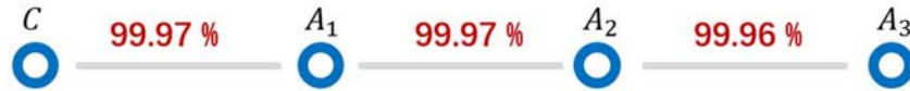
Figure 18: Illustrative BTA apportionment for a network topology with three radio sites connected to a remote aggregation point in a daisy-chain configuration
