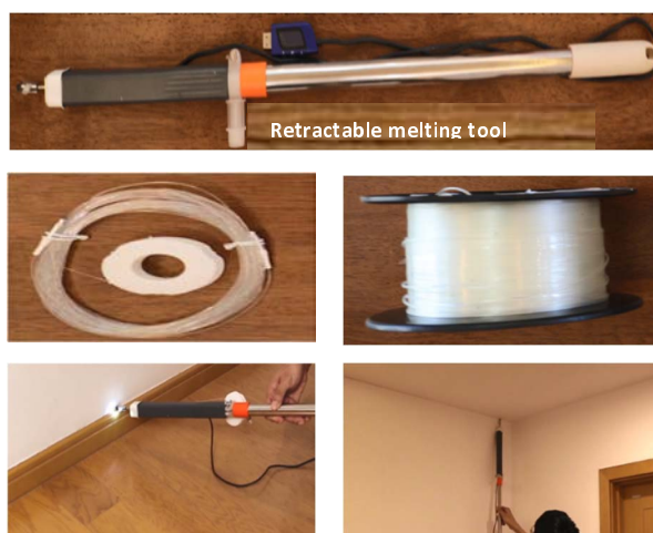
Figure 6.1: Deployment with hot-melt self-adhesive
