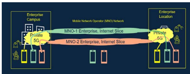
Figure 4.25.4-1: End-to-end QoS mobile service for Enterprise users
