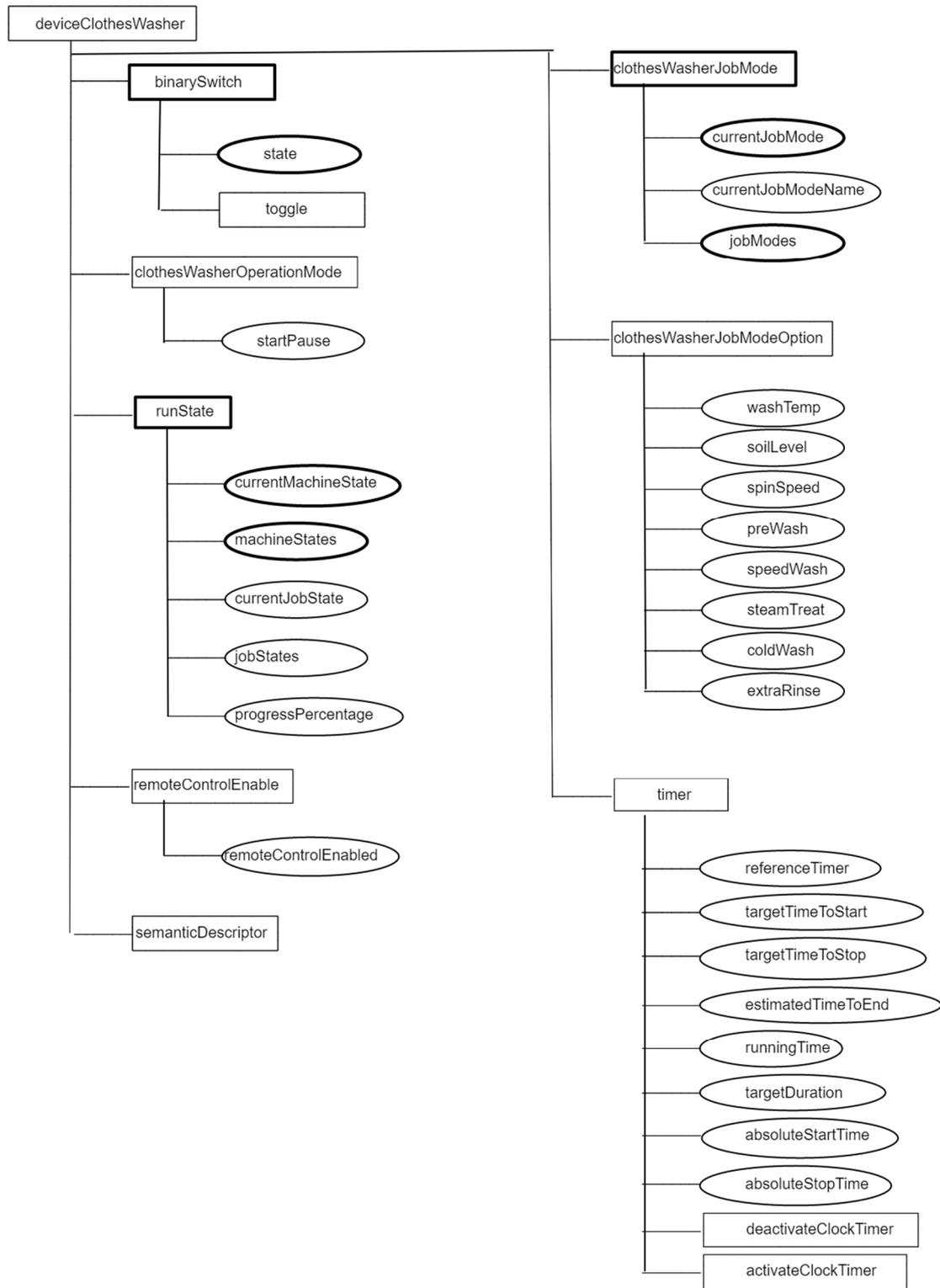
**Figure 4: SDT washing machine model**
