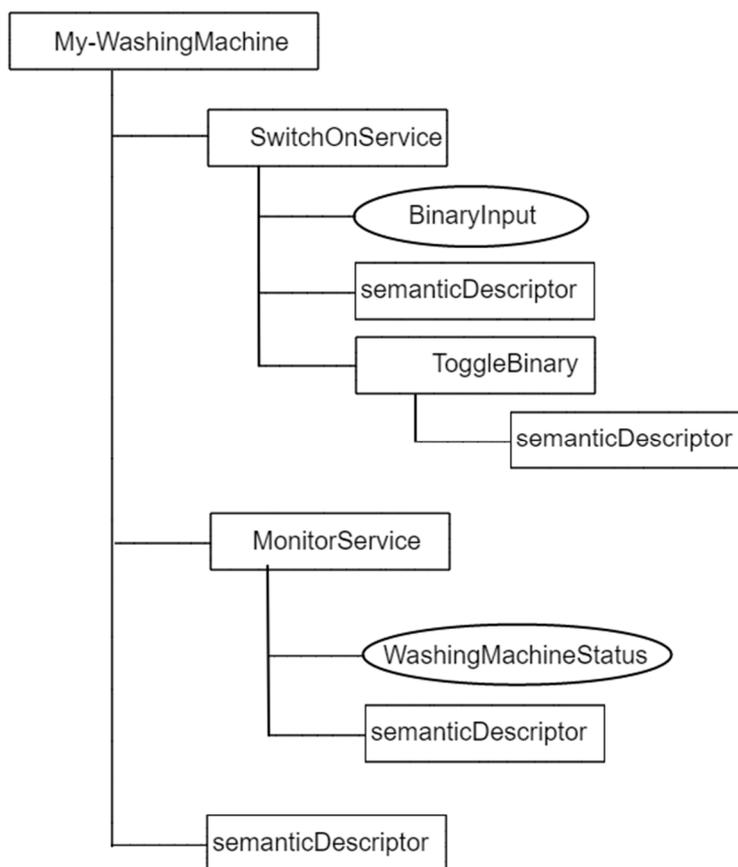
**Figure 5: SAREF washing machine model**
