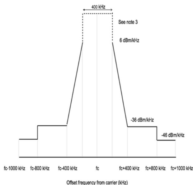
**Figure A.2: Proposed Spectral Mask**
