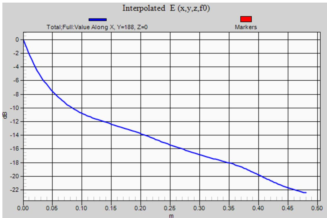
Figure B.2: Decay of field strength with distance
