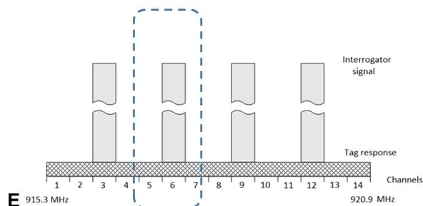
**Figure A.1: Graphical illustration of channel plan highlighted in EC implementing Decision (EU) 2018/1538 [i.4], Annex**
