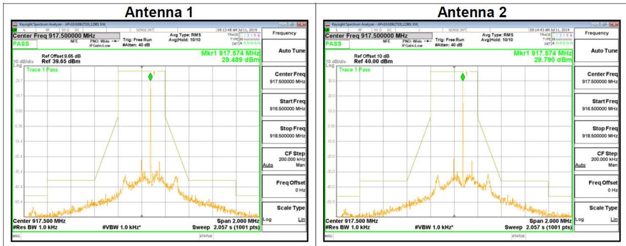
Figure B.1: Transmitter Spectrum Mask at 917,5 MHz
