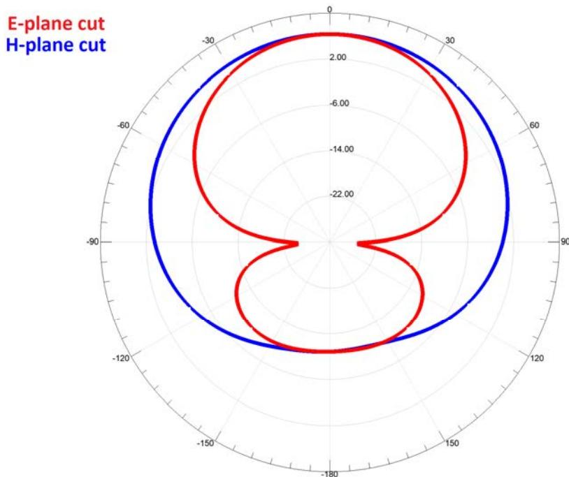
**Figure 1: Typical Antenna Radiation Pattern**
