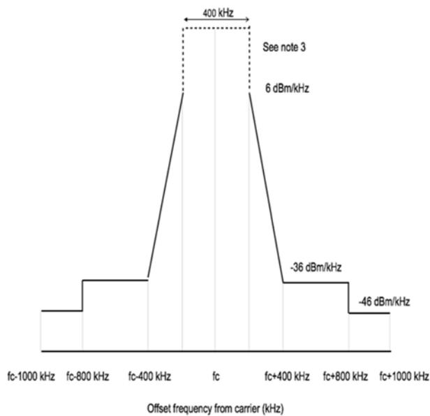
**Figure A.2: Proposed Spectral Mask**
