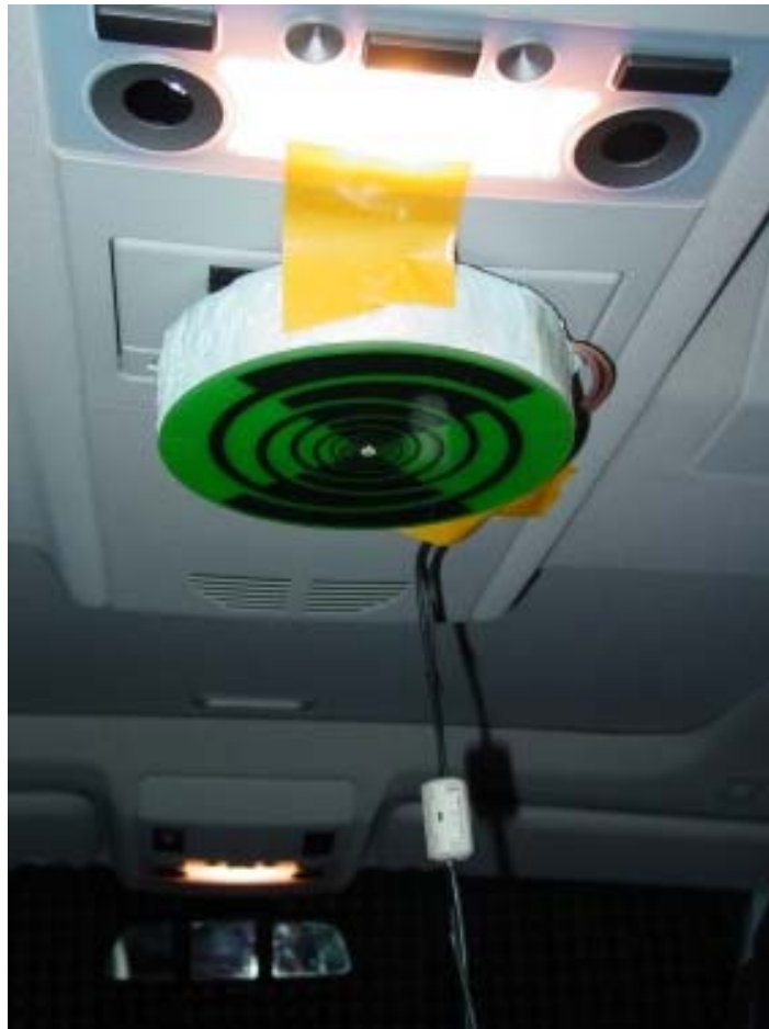
Figure 3: Installation of antenna for position 5 in Figure 2 (Source [i.45])
