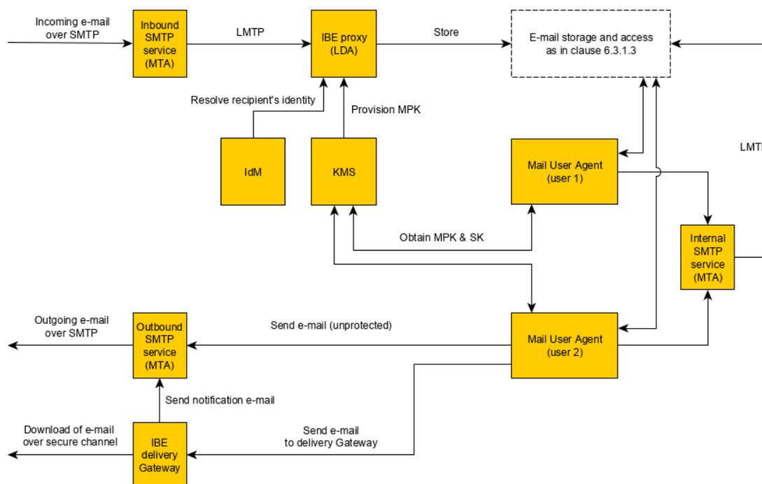
**Figure 13: Closed IBE cryptosystem supporting an e-mail domain, with options (a) and (b)**
