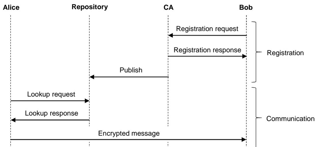
**Figure 5: Encrypted communication with a PKI**
