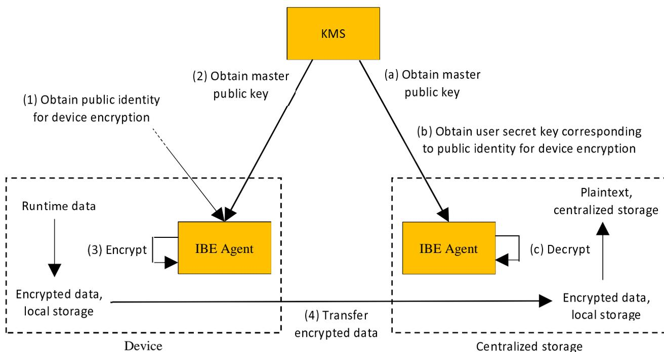
Figure 8: Locally irreversible encryption using IBE
