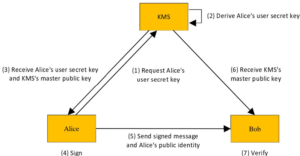
**Figure 4: Identity-based digital signature scheme**
