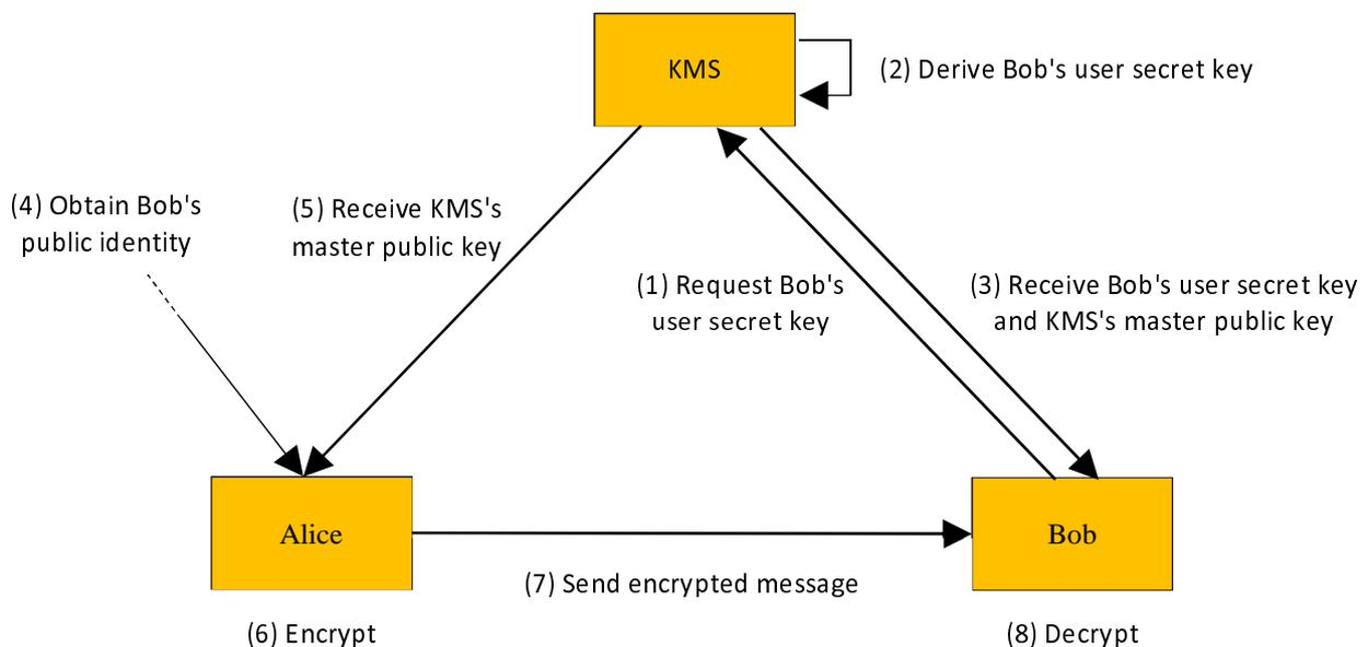
**Figure 2: General model of IBE cryptosystems**
