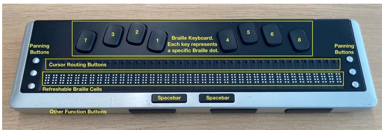
Figure 7: Common features of braille displays. Not all features will be available on all displays, but the device pictured represents a common feature set for desktop braille displays
