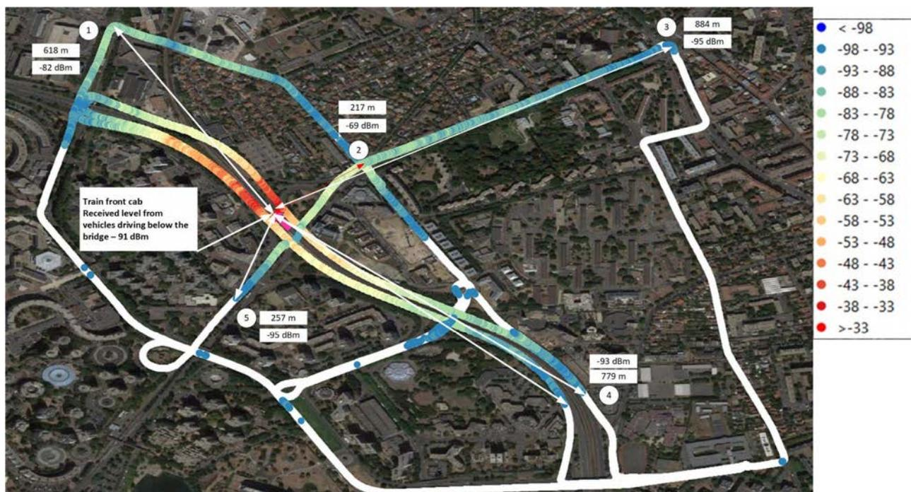
**Figure 62: Line 8 section 2-3 level received from two vehicles by the Train front cab at position 4 (Map Source Google Earth: © Google)**
