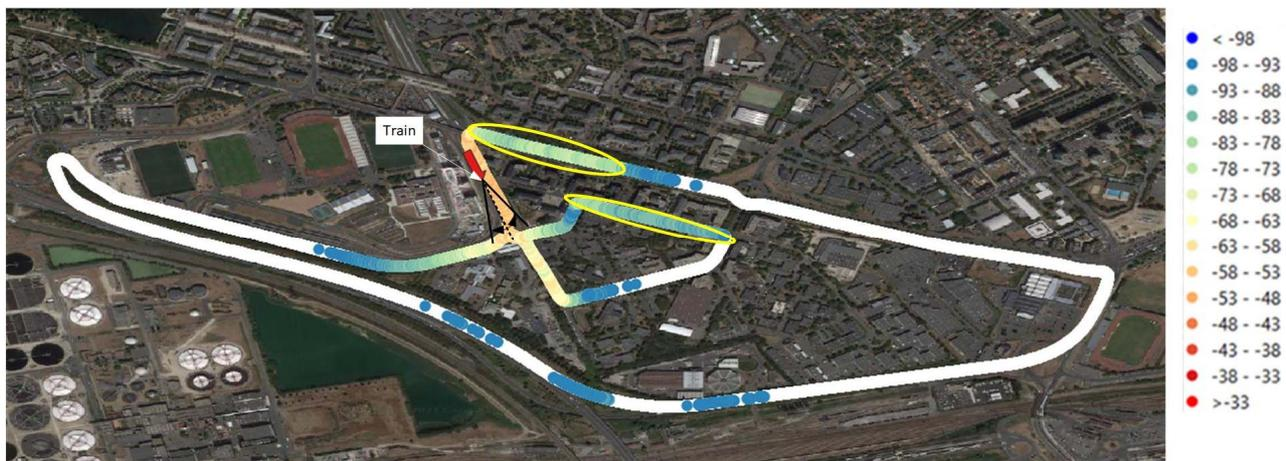
**Figure 53: Line 8 section 1 Train position 2 level received from vehicles for EIRP 33 dBm/10 MHz (Map Source Google Earth: © Google)**
