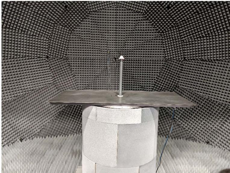
**Figure A.16: Placement of the antenna in the centre of the EMSL positioned over the metallic support to simulate the roof of the vehicle**
