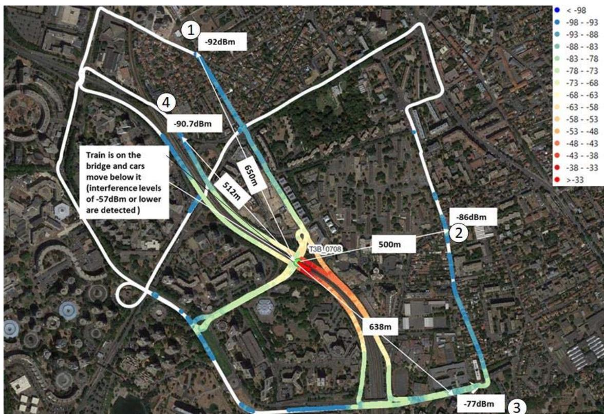
**Figure 59: Line 8 section 2-3 level received from two vehicles by the Train rear cab at position 3 (Map Source Google Earth: © Google)**
