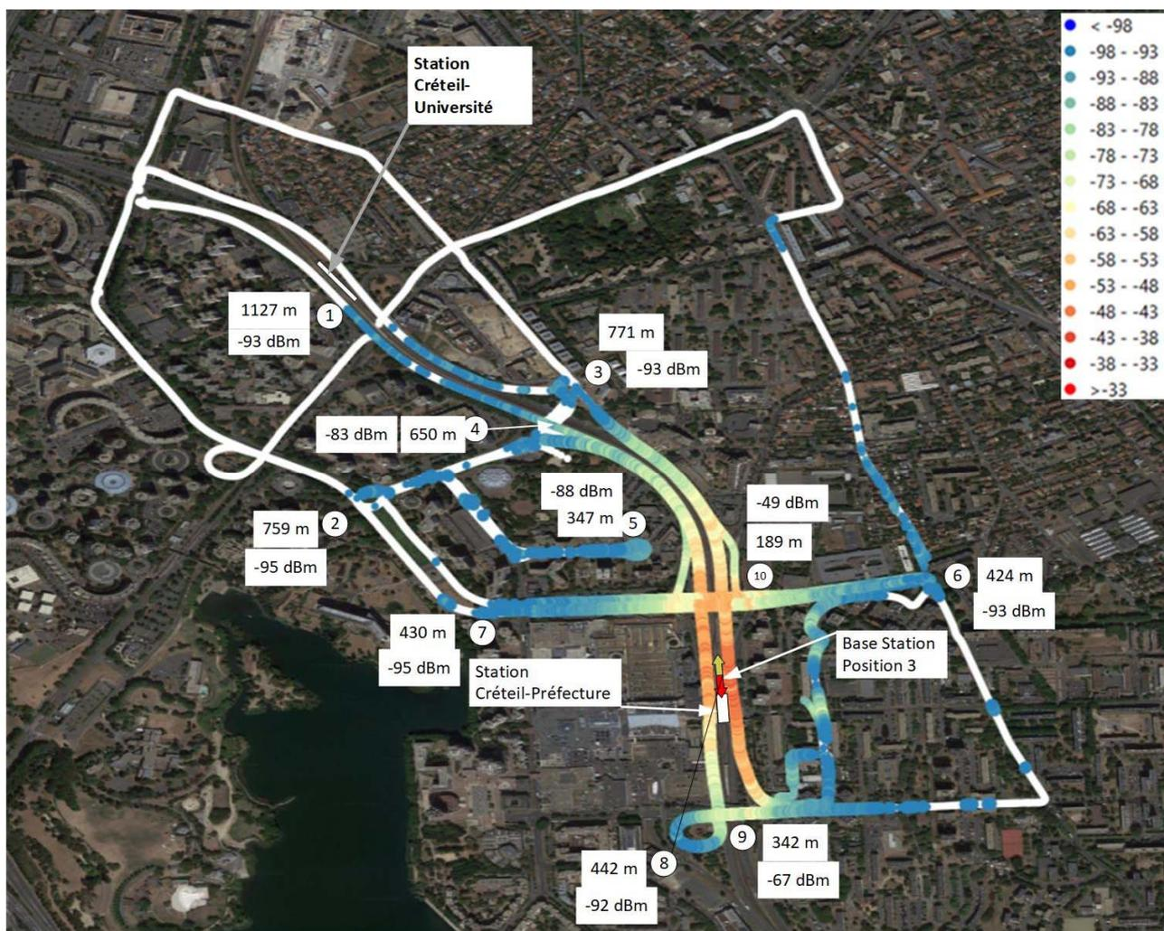
**Figure 65: Line 8 section 2-3 level received from two vehicles by base station at position 3 (Map Source Google Earth: © Google)**
