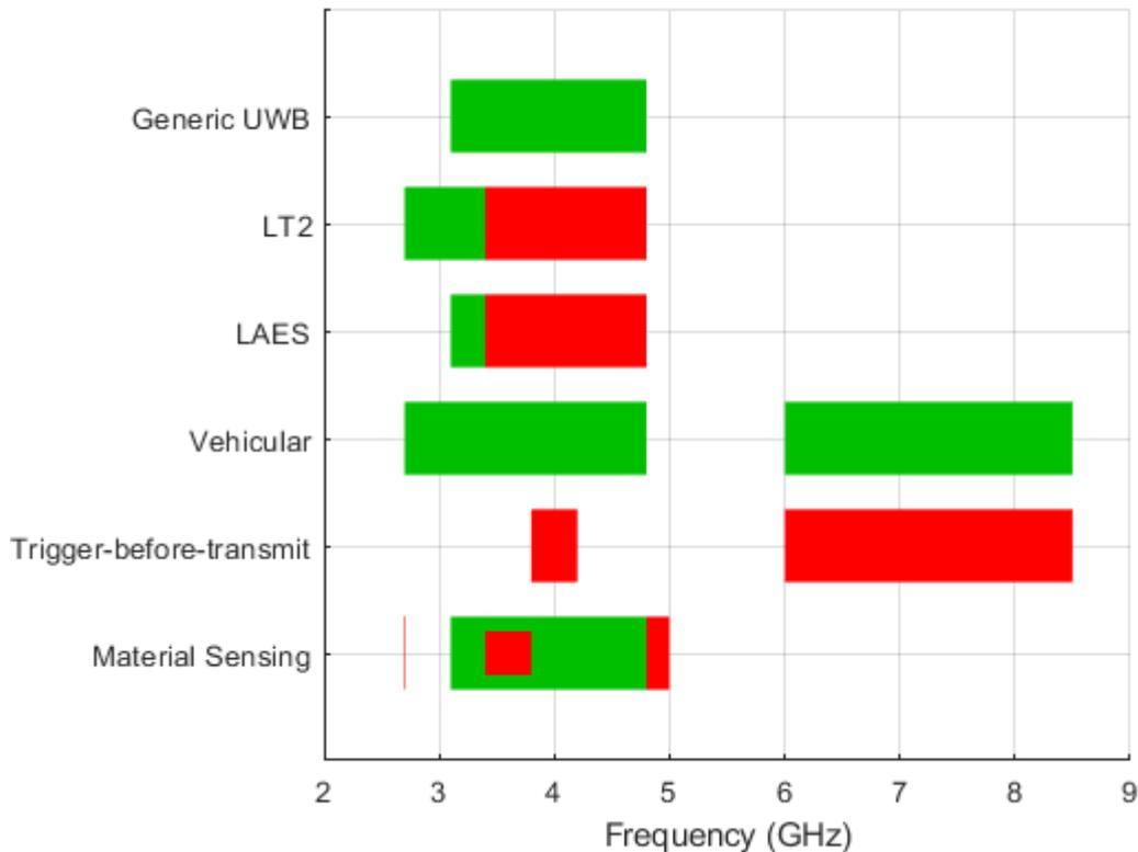
Figure 1: Duty cycle applicability in UWB regulations
