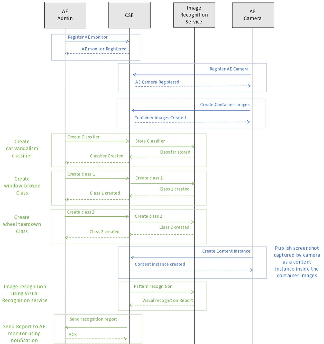
Figure 6: Sequence diagram of Use Case 2
