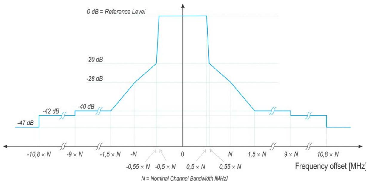
**Figure 3: Transmit spectral power mask**
