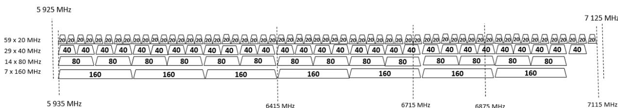
**Figure 2: IEEE P802.11ax [i.20] channel arrangement for the 6 GHz band**
