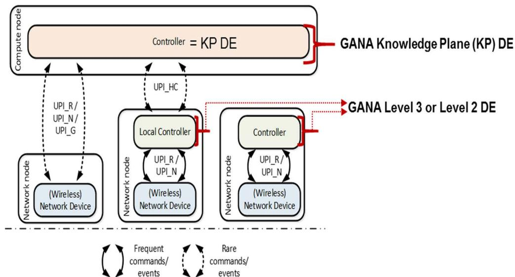
**Figure 19: Various implementations scenarios that can be considered in implementing GANA DEs as controllers**
