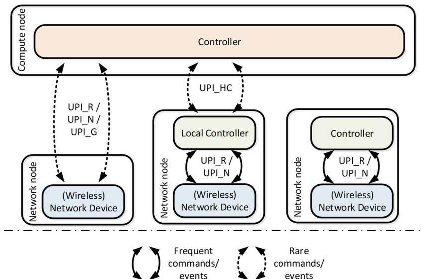
NOTE: Global controllers (left) handle rare events and commands while local controllers (right) are able to handle frequent commands and events. In hierarchical control (middle) there are two control loops, i.e. outer and inner.
