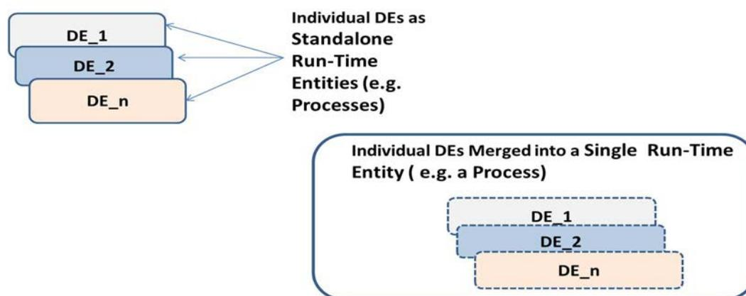
**Figure 20: Illustration of possible approach to implementing GANA Levels 2, 3 and 4 DEs at run-time (extract from ETSI TS 103 195-2 [i.9])**
