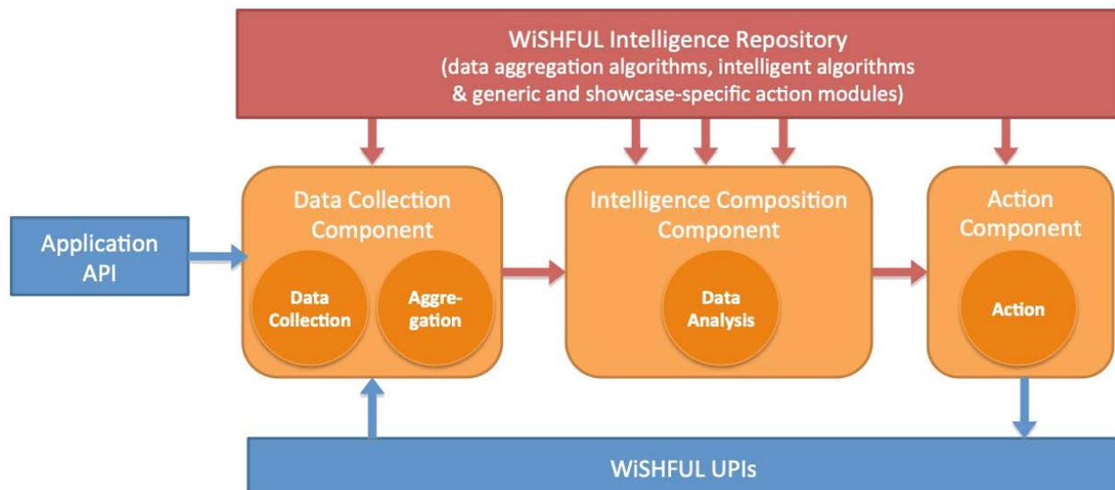
**Figure 8: Conceptual framework for enabling intelligence in the WiSHFUL architecture**
