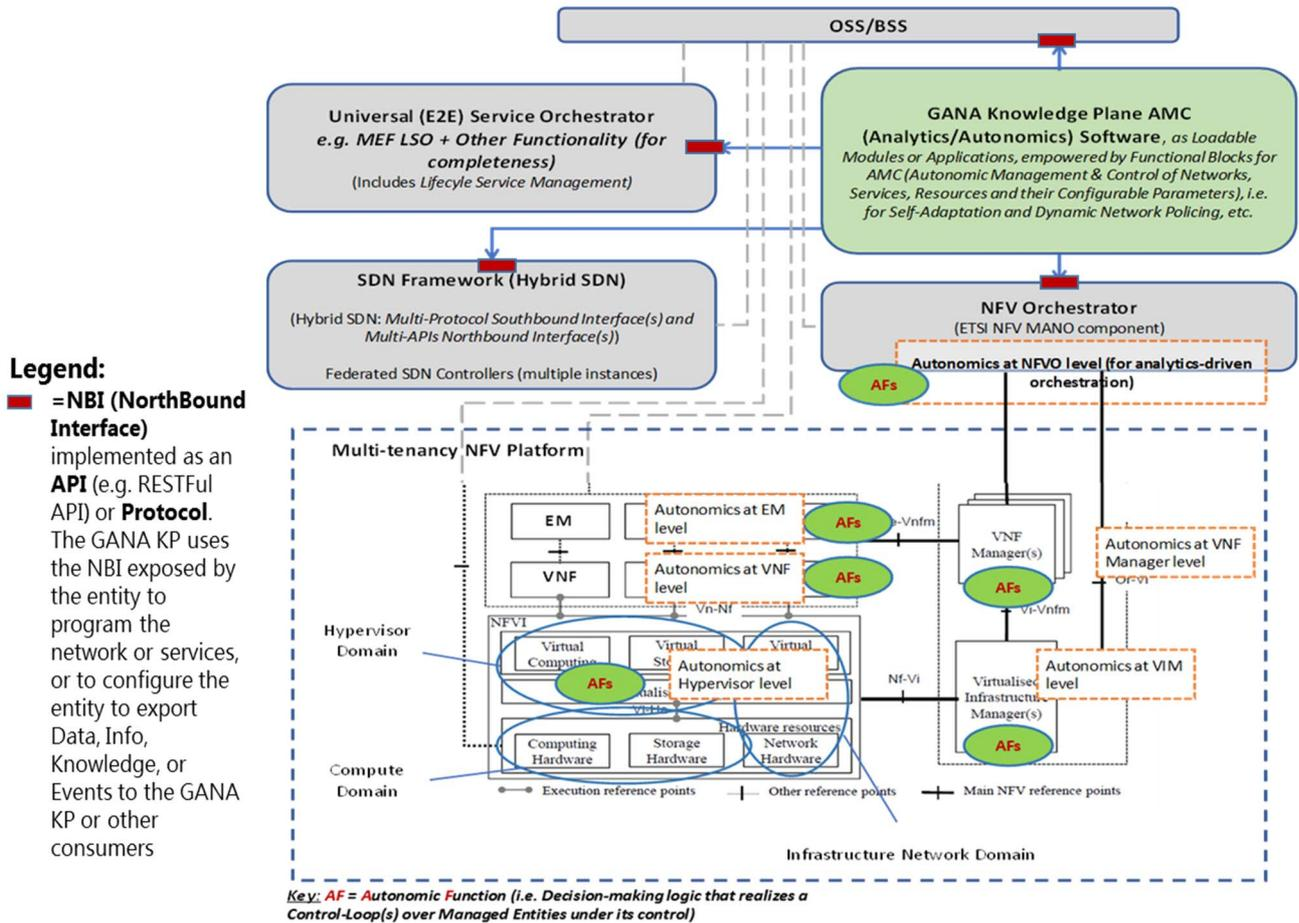
Figure 12: Multi-Layer Autonomics and the integration of the GANA Knowledge Plane with Orchestrators, SDN Controllers, NFV, and OSS/BSS systems
