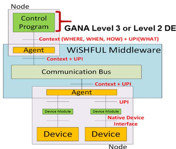
**Figure 16: A GANA level 2 or Level 3 DE is treated as a Local Control Program in the WiSHFUL Framework (with additional insights concerning contexts)**
