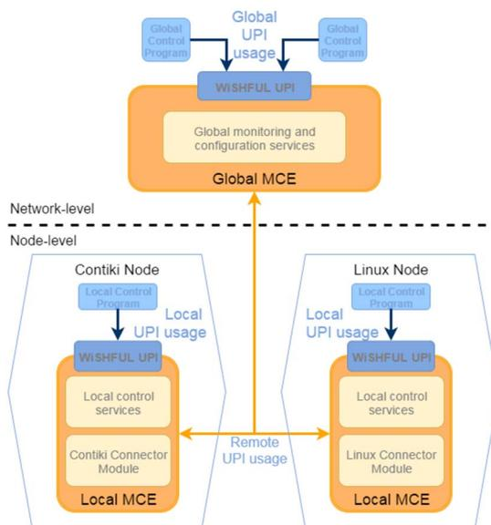
**Figure 6: Overview of the components in the general WiSHFUL architecture**
