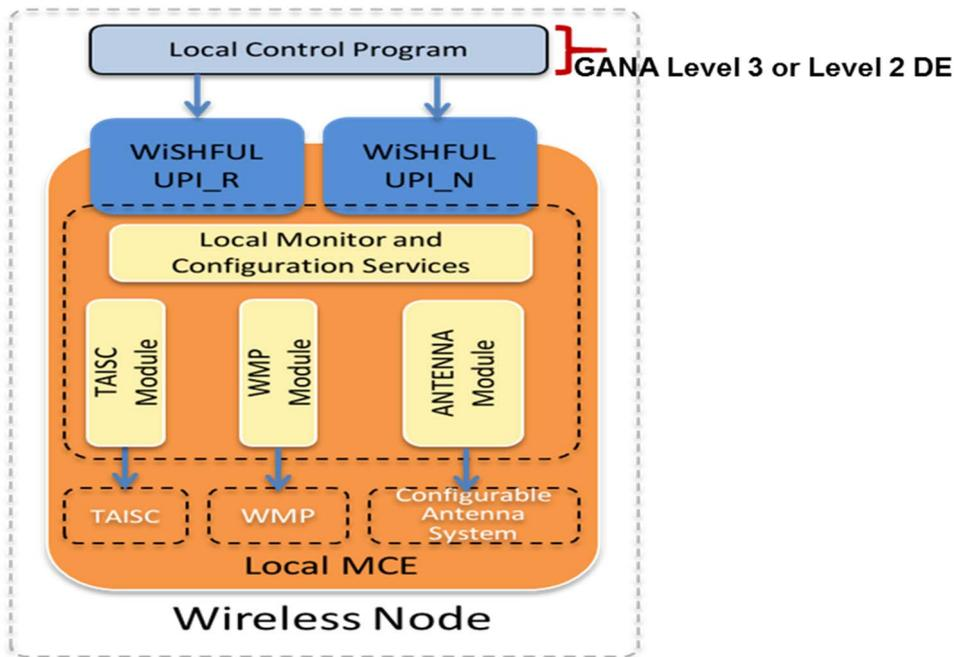
Figure 14: A GANA level 2 or Level 3 DE is Local Control Program in the WiSHFUL Framework
