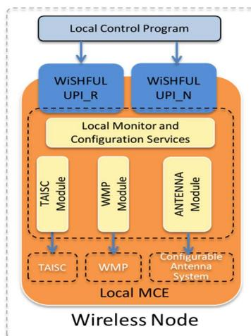
**Figure 3: Example of wireless node supporting three different platforms**
