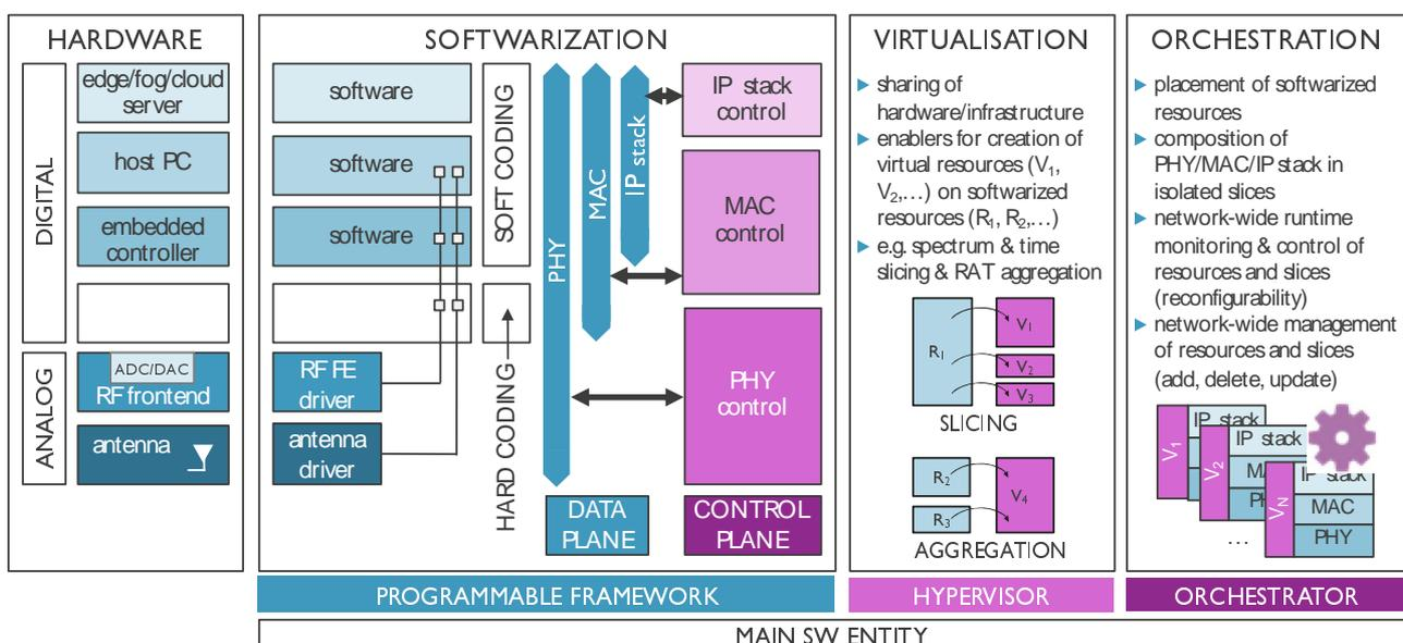
**Figure 9: Illustration of Softwarization, virtualization and orchestration principles in the H2020 ORCA project**
