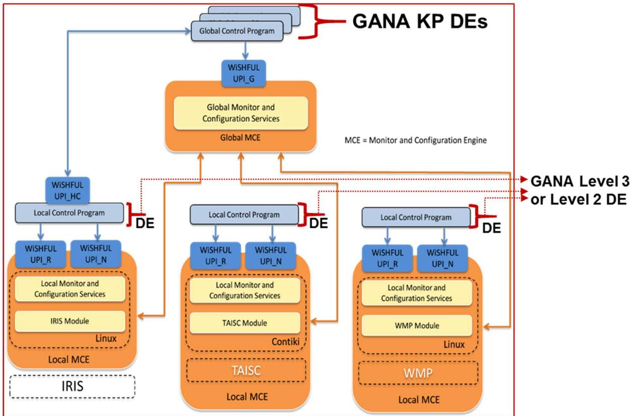
**Figure 17: A GANA level 2 or Level 3 DE is treated as a Local Control Program in the WiSHFUL Framework, and a GANA Knowledge Plane (KP) Level DE is a Global Control Program in the WiSHFUL Framework**
