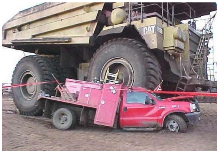
Figure A.7: Collision avoidance for large construction vehicle (source: Bosch)
