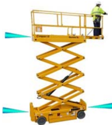
Figure A.9: Work platform: surveillance of "blind spots" (source Bosch)
