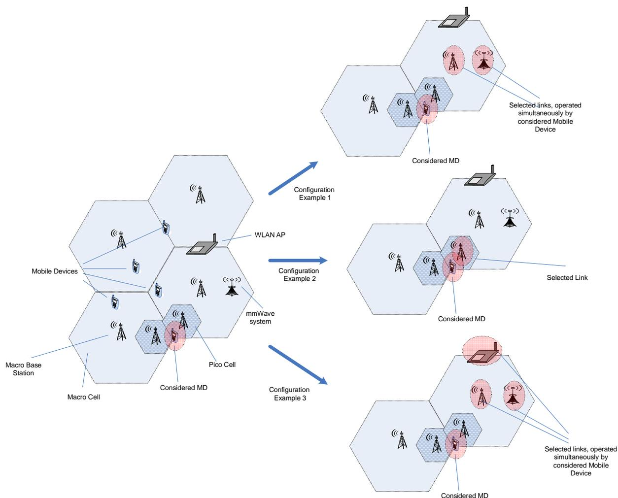
**Figure 2: Scenario Illustration "Optimized Configuration selection in a Heterogeneous Radio Context" - the best combination is identified comprising of a single link or multiple links being operated simultaneously**
