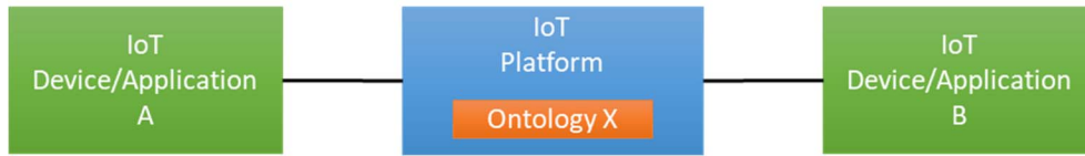
Figure 3: Configuration CFG-02 - Two IoT devices/Applications on a single IoT platform
