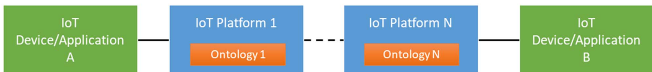
Figure 7: Configuration CFG-06 - Multiple IoT devices/Applications on multiple IoT platforms using different ontologies
