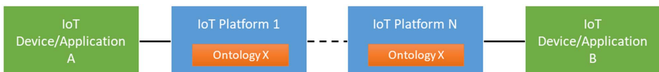
Figure 5: Configuration CFG-04 - Two IoT devices/Applications on multiple IoT platforms using a common ontology
