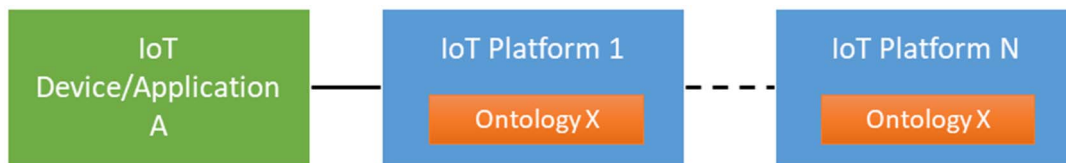
Figure 4: Configuration CFG-03 - Single IoT devices/Applications on multiple IoT platforms
