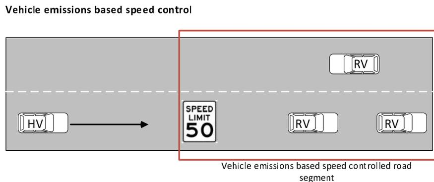
**Figure 2: Use-case vehicle emissions based speed control**
