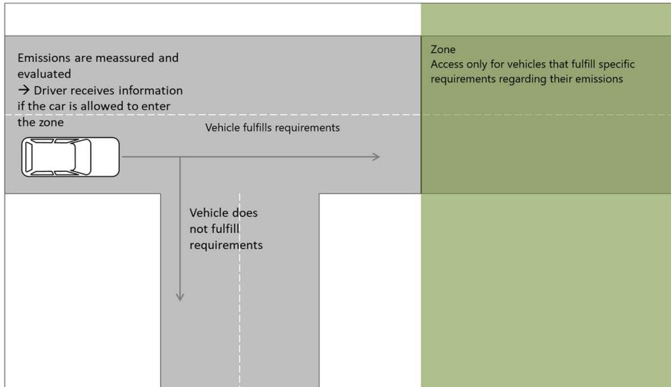
Figure 4: Illustration use-case access restriction based on vehicle emission types
