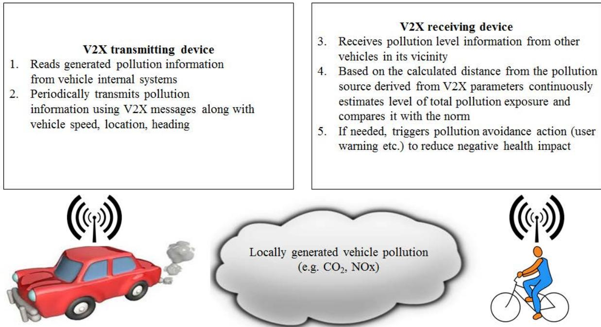
**Figure 1: Simplified diagram of the V2X based emissions crowdsourcing approach**
