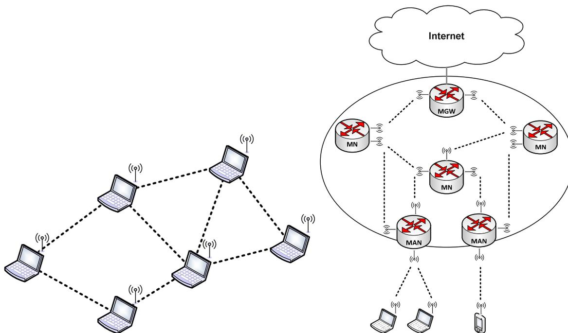
**Figure 7: Common aspects between Ad-hoc (left) and mesh networks (right) include multi-hop wireless transmission**
