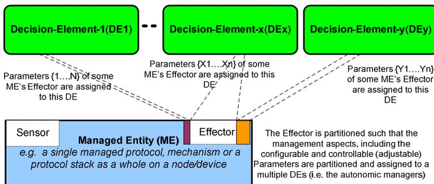
**Figure 5: Parameter mapping Case 2: an ME with an effector partitioned such that varying parameter sets are assigned to different DEs)**
