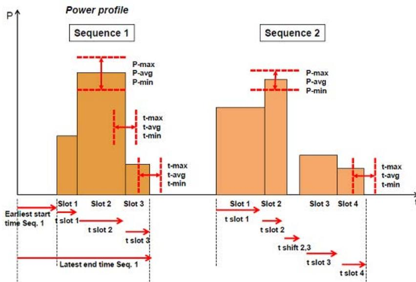
Figure 8: EEBus representation of power profile and related concepts
