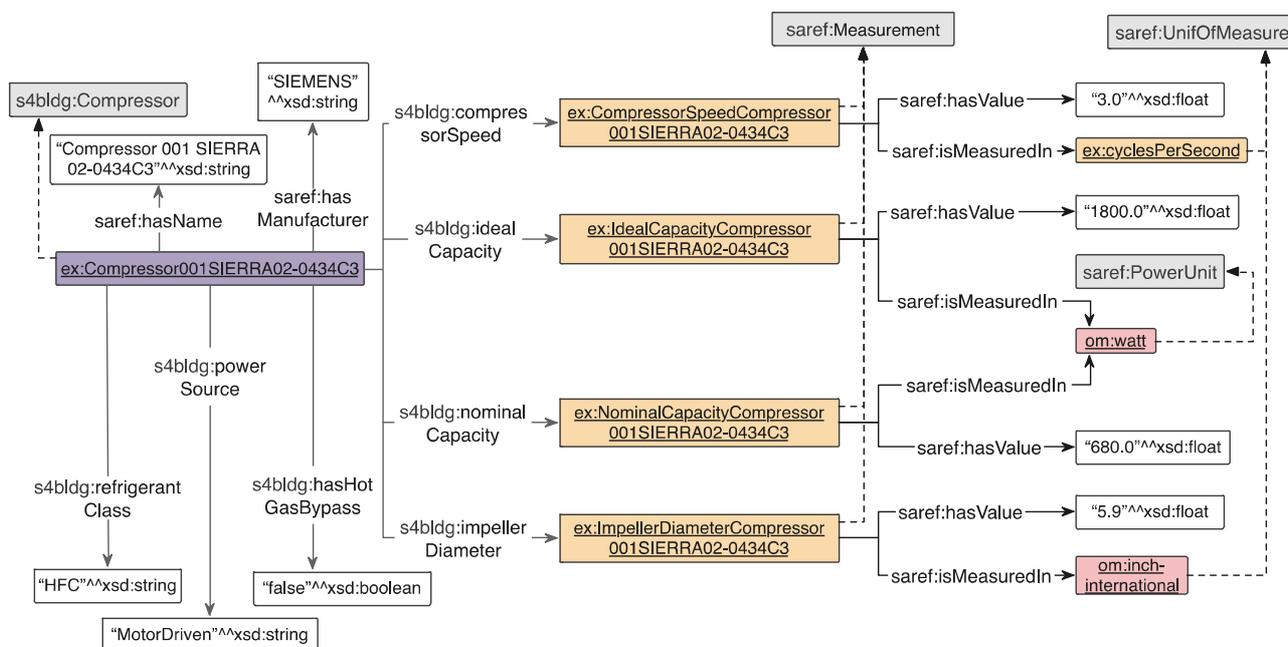
Figure 13: Compressor description example
