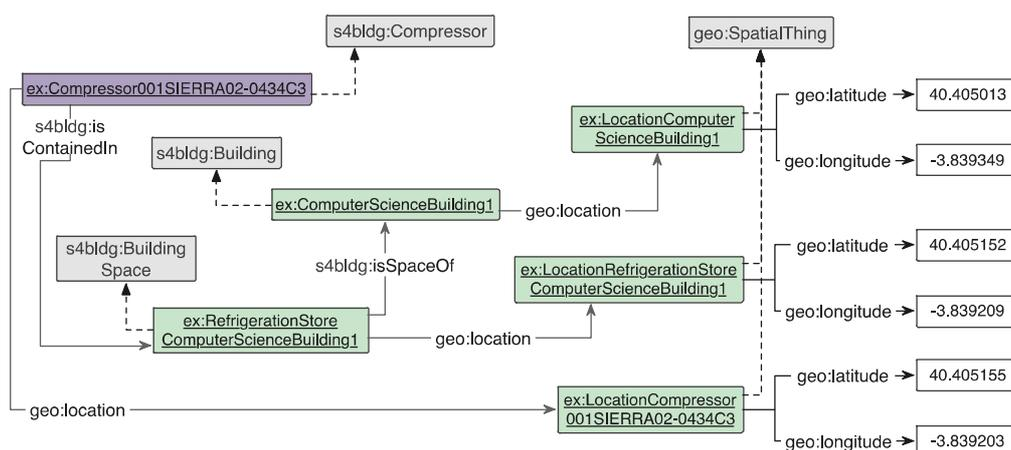
**Figure 14: Compressor location example**
