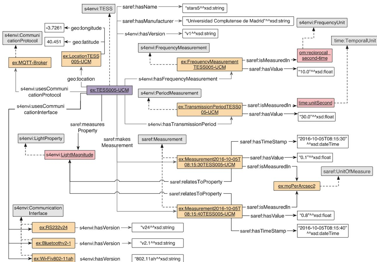
Figure 11: Photometer TESS description example
