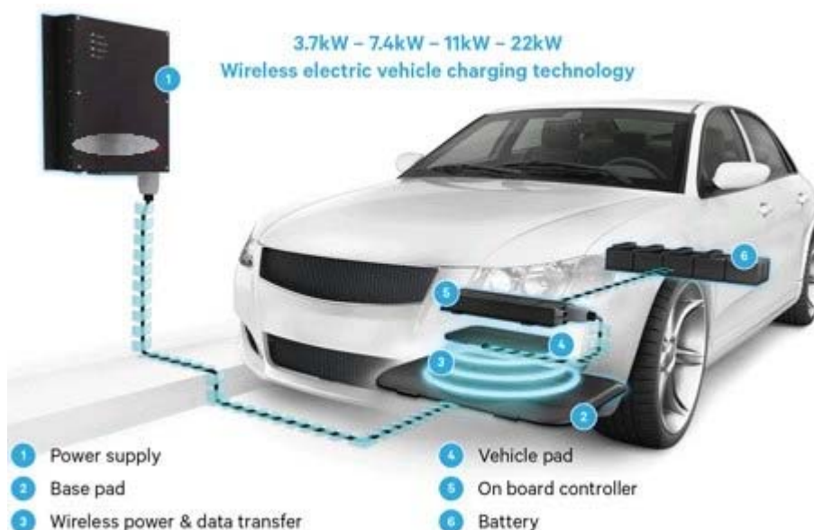
Figure 19: Wireless electric vehicle charging system (with permission of Qualcomm)
