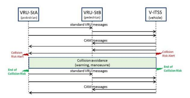
Figure 10: Flow diagram for UC-B2-alt - VRU crossing on a bridge
