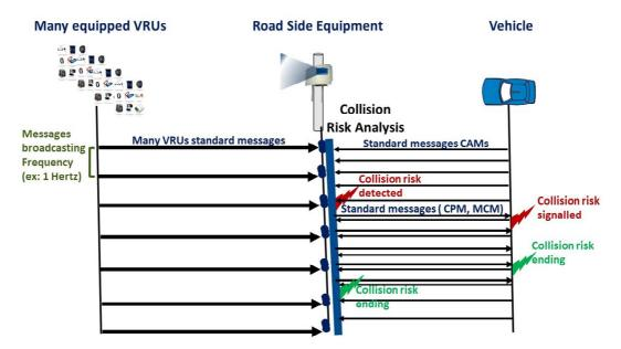
Figure 33: Alternative flow diagram for UC-F1 - Many VRU in a protected area
