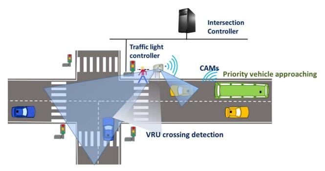
Figure 26: Illustration of UC-D3 - VRU at a pedestrian crossing with a traffic light
