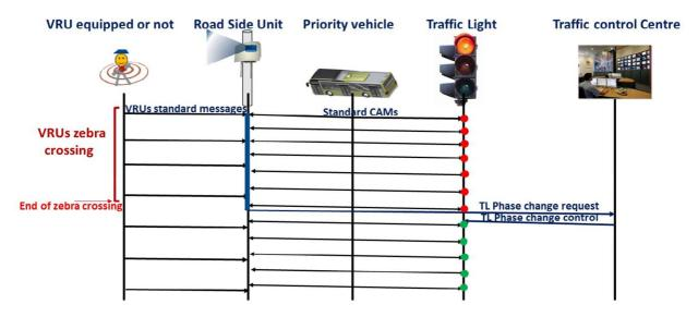
Figure 25: Flow diagram for UC-D3 - VRU at a pedestrian crossing with a traffic light
