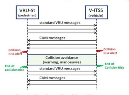
Figure 8: Flow diagram for UC-B2 - VRU at crossroad
