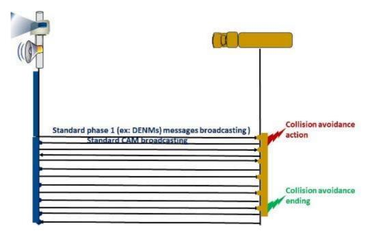
Figure 20: Flow diagram for UC-D1: Few VRU in a protected area
