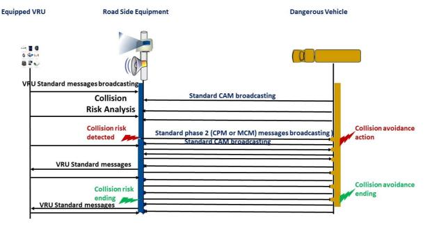
Figure 21: Alternate flow diagram for UC-D1: few VRU in a protected area
