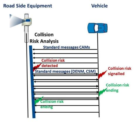
Figure 32: Flow diagram for UC-F1 - Many VRU in a protected area
