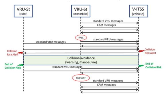
Figure 12: Flow diagram for UC-B3 - Rider is separated from his motorcycle
