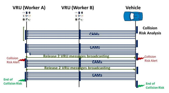
Figure 6: Alternative flow diagram for UC-B1 - Active roadwork
