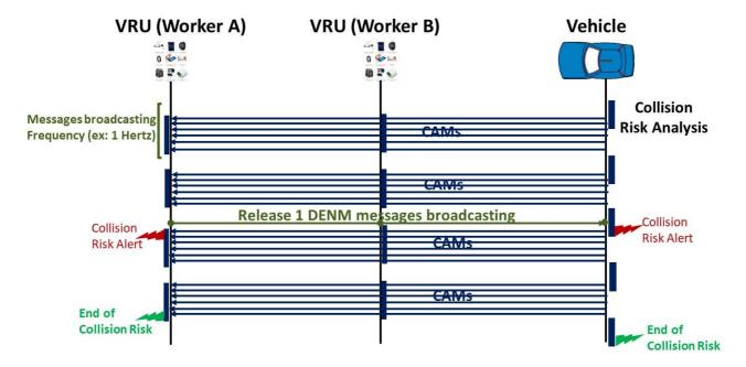
Figure 5: Flow diagram for UC-B1 - Active Roadwork
