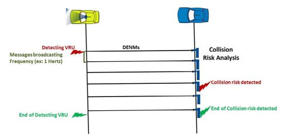
Figure 18: Flow diagram for UC-C1: VRU hidden by an obstacle
