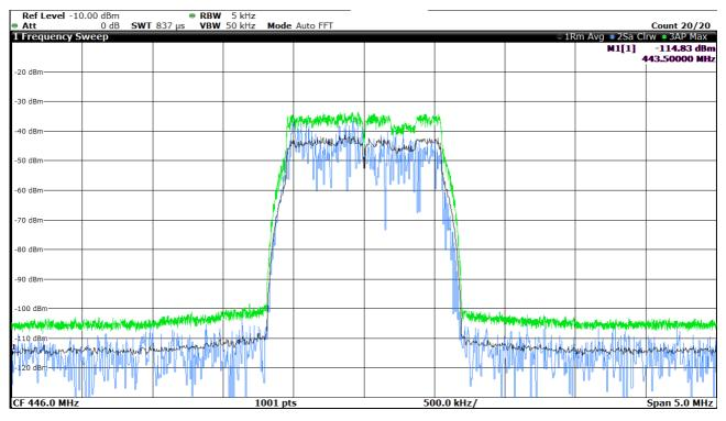
Figure H.8: 1,4 MHz LTE Signal E-TM1.2
