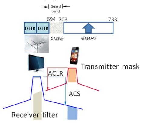
Figure E.1: Illustration of the interference mechanism and the related characteristics
