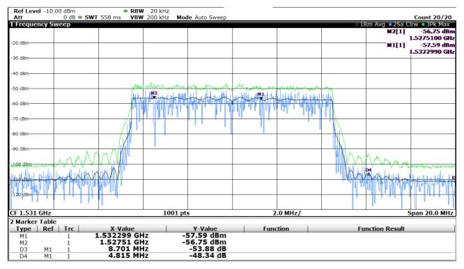
Figure H.1: E-TM1.1 signal, -33 dBm mean power
