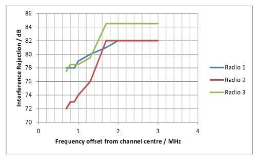
Figure H.17: Comparison of results for PMR Radios 1, 2 and 3 with E-TM2 interferer
