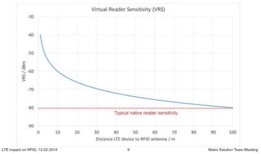
Figure G.3: Loss in sensitivity loss of interrogator due to LTE OOB emissions
