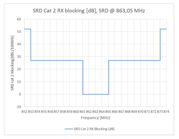
Figure C.1: Blocking specification of a 100 kHz wide category 2 SRD receiver in ETSI EN 300 220-1
