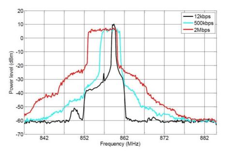
Figure G.2: In-band and out-of-band power levels (RBW of 180 kHz)
