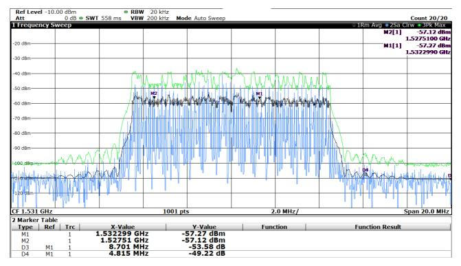
Figure H.3: E-TM2 signal ("idle mode"), -33 dBm mean power, Slow sweep
