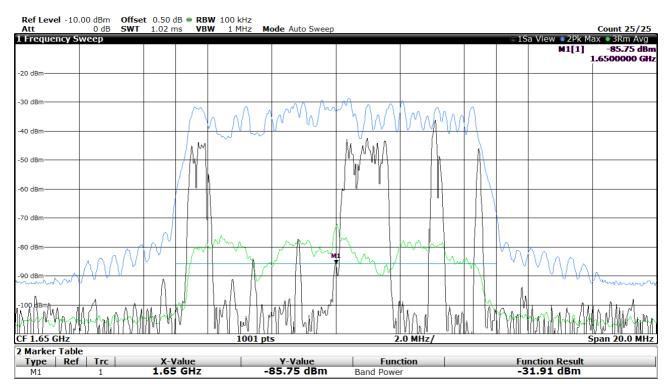
Figure H.4: E-TM2 signal ("idle mode"), fast sweep
