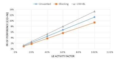
Figure F.1: Probability of interference for Cat.2 SRD Metering
