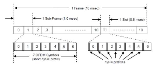
Figure B.1: The structure of a LTE frame
