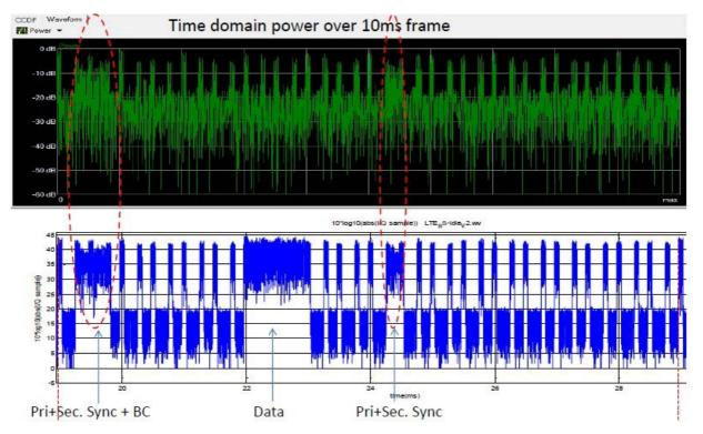
NOTE: The recorded signal presents a longer burst corresponding to the transmission of user data. (Source: Sony Europe).
