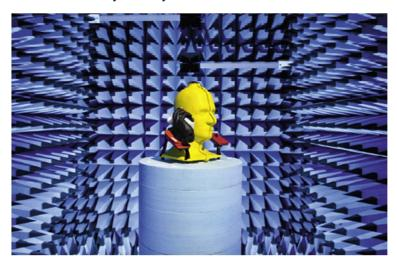
Figure F.3: TRP test set up in an anechoic chamber
