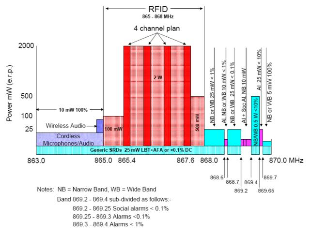
Figure G.1:Short range Devices frequency plan according the EC decision [i.3] related to Short Range Devices
