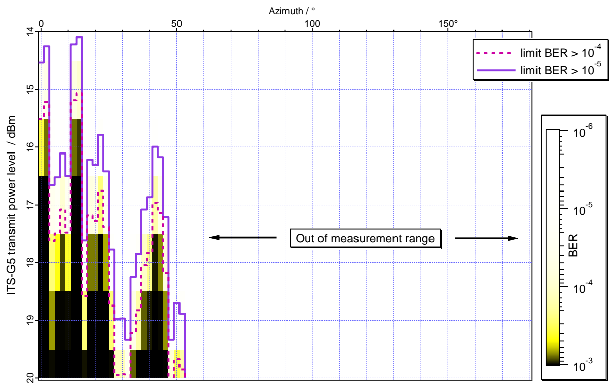
Figure A.20: OBU12 at sensitivity limit (DSRC incident power level -49,2 dBm), raw BER data, TD_COEX_OBU_01, test run 4
