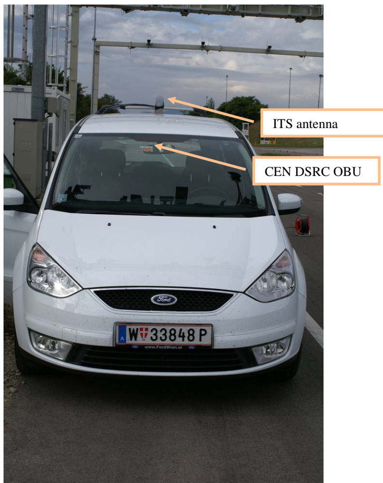
Figure 53: Mounting of OBU and ITS antenna
