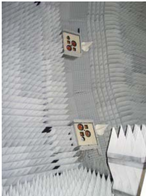
Figure 50: Chamber's movable antenna system
