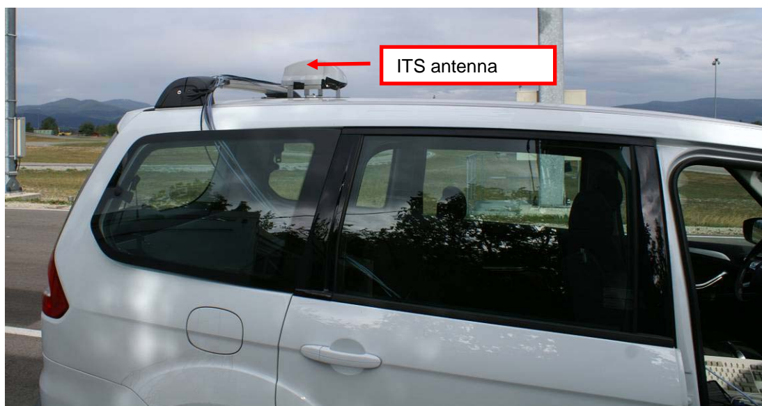
Figure 54: Mounting of ITS antenna
