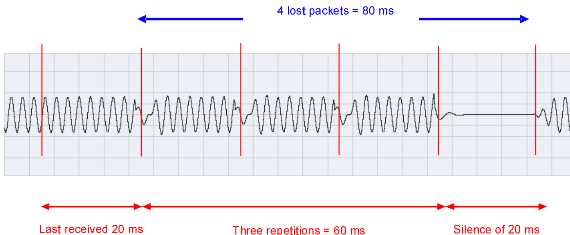
Figure 6: Example of PLC behaviour testing with a 440 Hz sinewave
