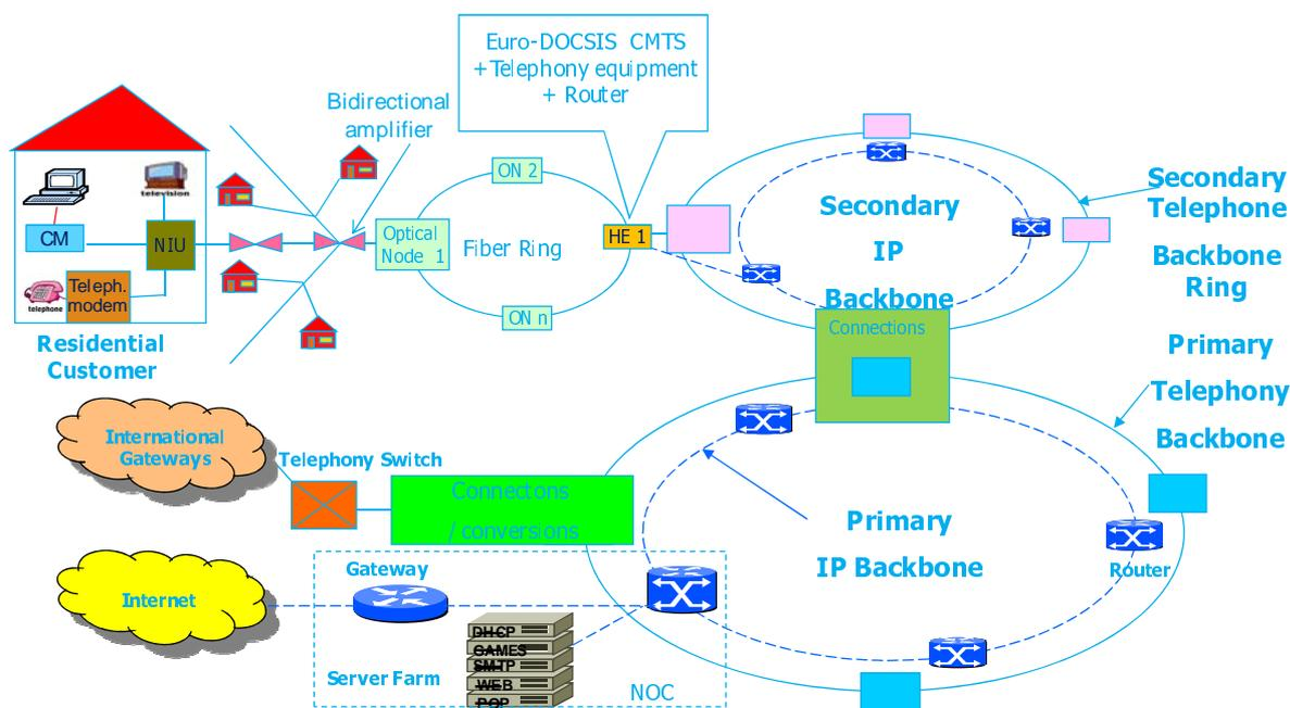
**Figure 9: HFC and backbone network topology of the cable operator's network**
