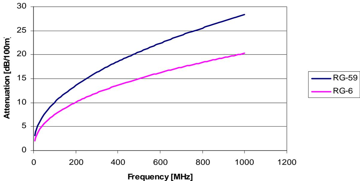
**Figure 2: Frequency dependence of the attenuation of two types of coaxial cables**
