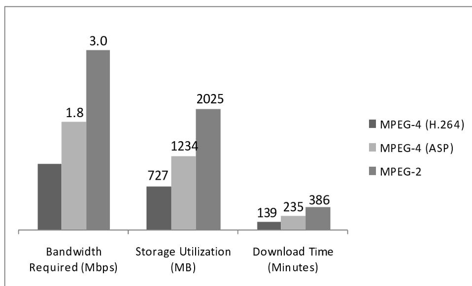
**Figure 15: Performance comparison of MPEG-2 and MPEG-4 compression for a 90-minute DVD-quality movie (download time at 700 kbps)**
