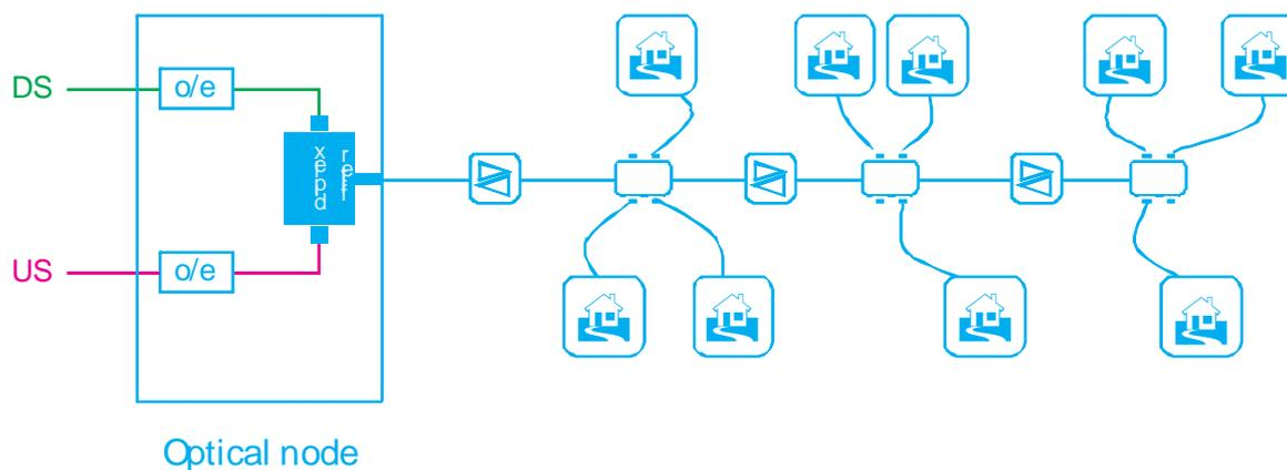
**Figure 5: Tree-and-branch HFC network topology**
