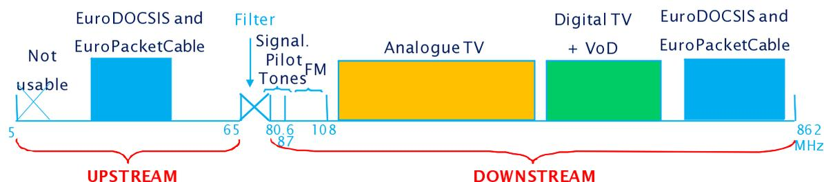
**Figure 12: Down- and upstream spectrum in an HFC network**
