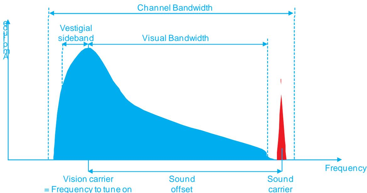
**Figure 17: RF spectrum of an analogue TV signal**
