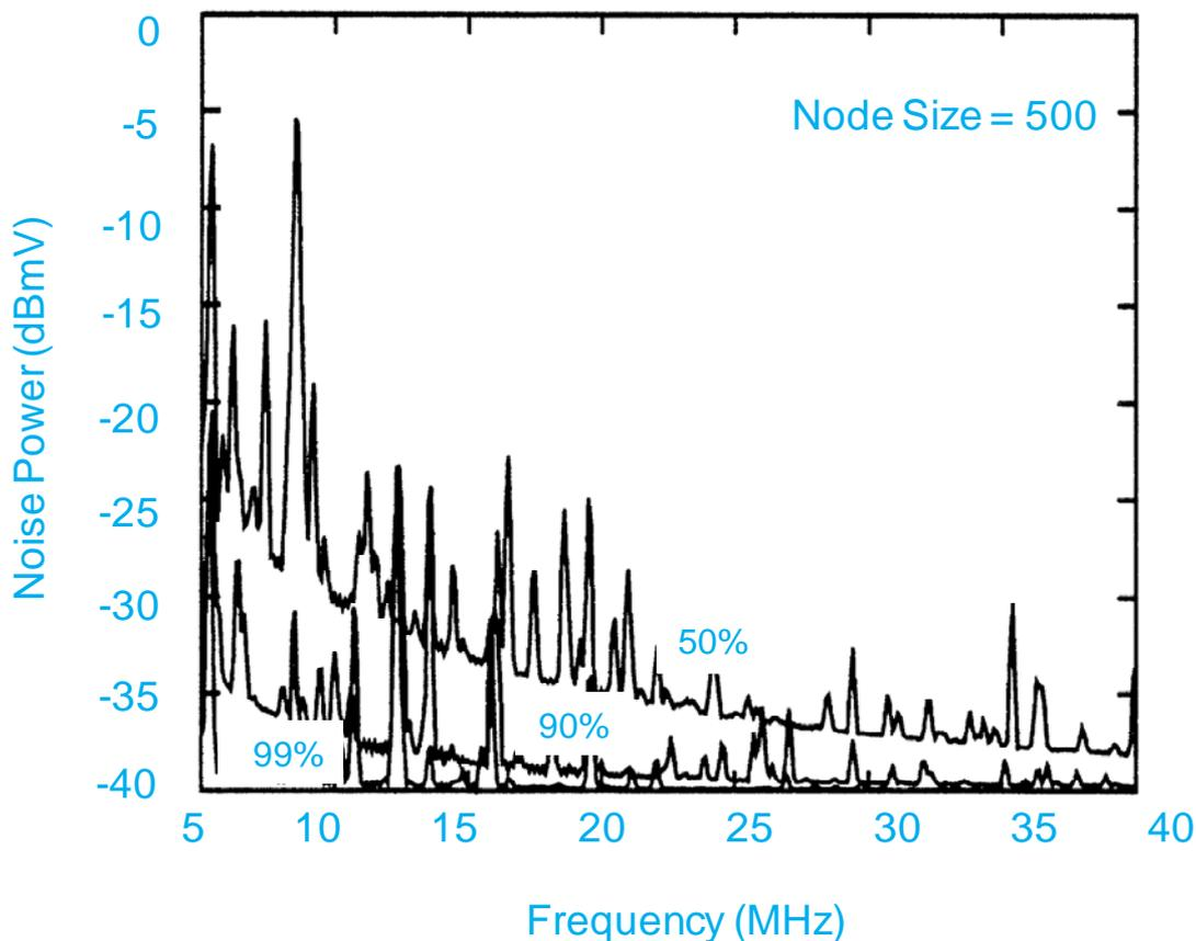
**Figure 13: Example of the upstream ingress noise spectrum**
