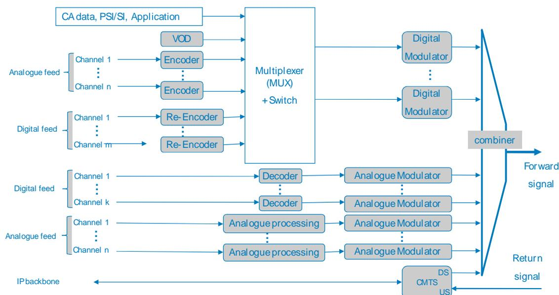
**Figure 16: Block diagram of the television and internet part of the cable headend**
