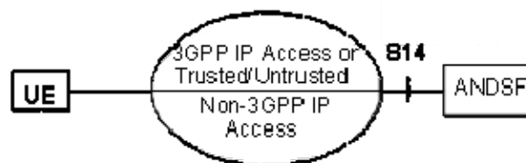
Figure 19: 3GPP Architecture for Access Network Discovery and Support Functions [i.1]
