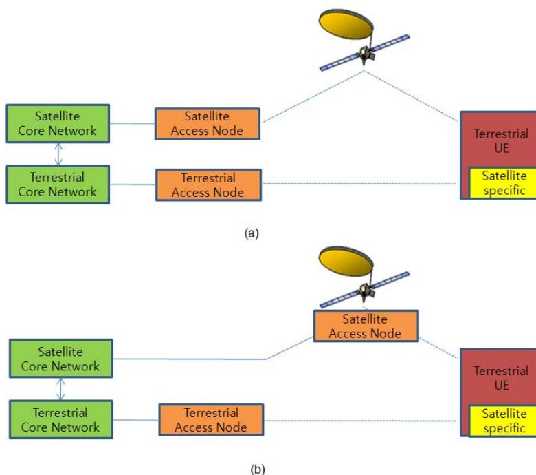
**Figure 7.2: Hybrid terrestrial and satellite system architecture**
