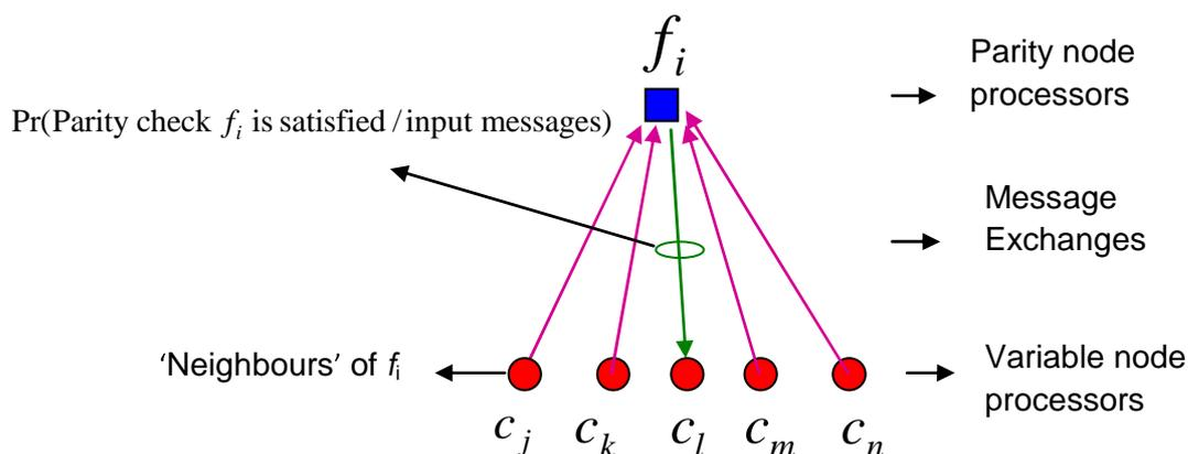
**Figure E.5: Second Pass in the BP Algorithm**
