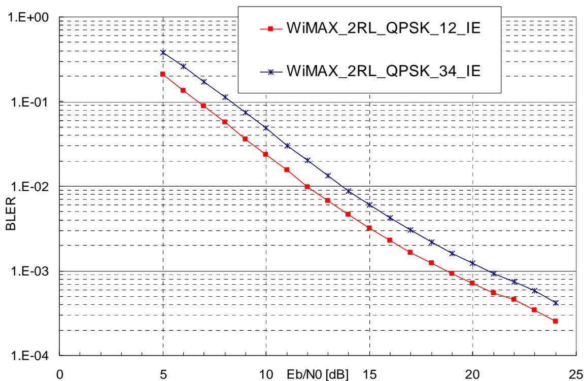
Figure I.31: BLER vs.  $E_b/N_0$  [dB], WiMAX Two-Way RL PHY configurations - Ideal Estimation
