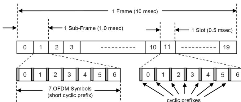
Figure H.11: First type of frame structure (compatible both with FDD and TDD modes)
