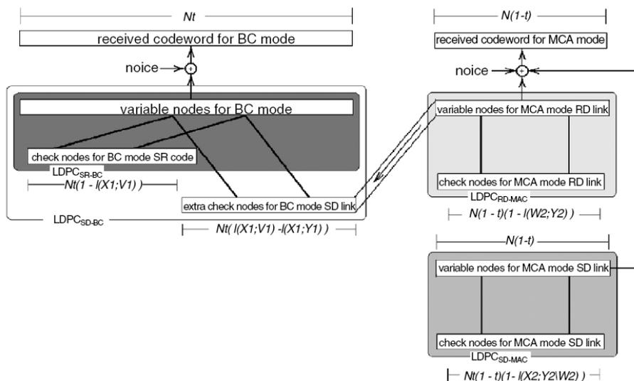
Figure L.7: LDPC Code Structure for  $\rho = 0$
