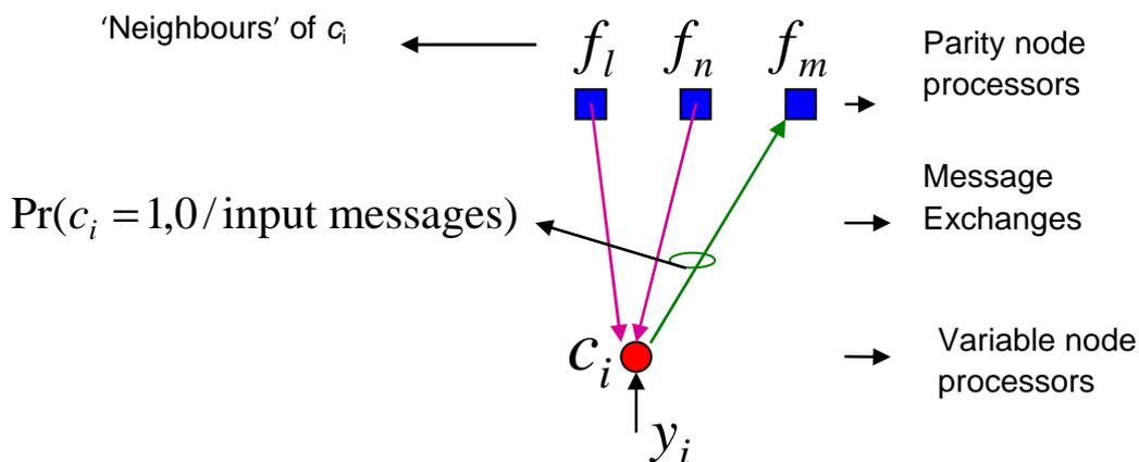
**Figure E.4: First Pass in the BP Algorithm**
