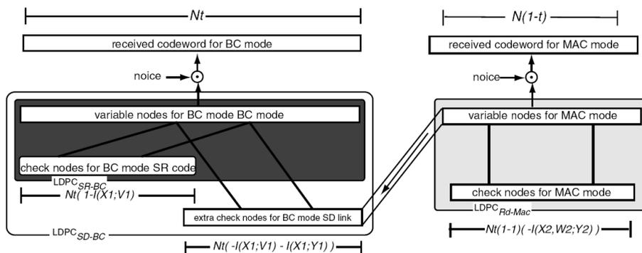
Figure L.6: LDPC Code Structure for  $\rho = 1$
