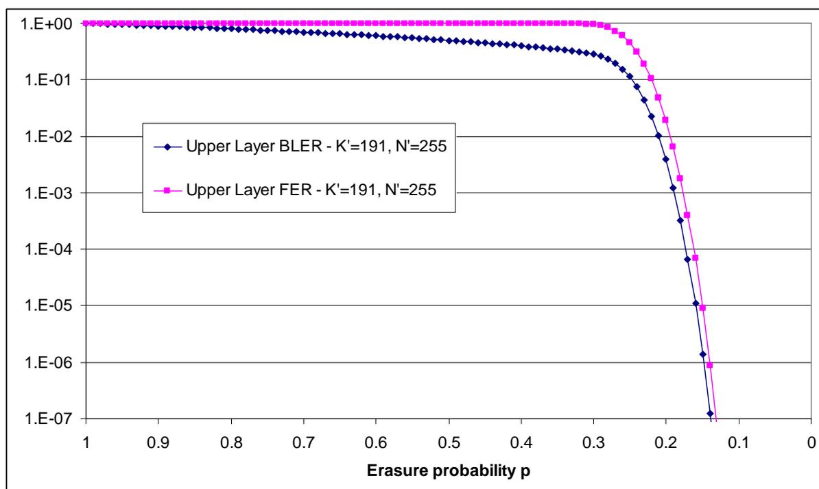
Figure I.37: Upper Layer BLER over the BEC. CASE A
