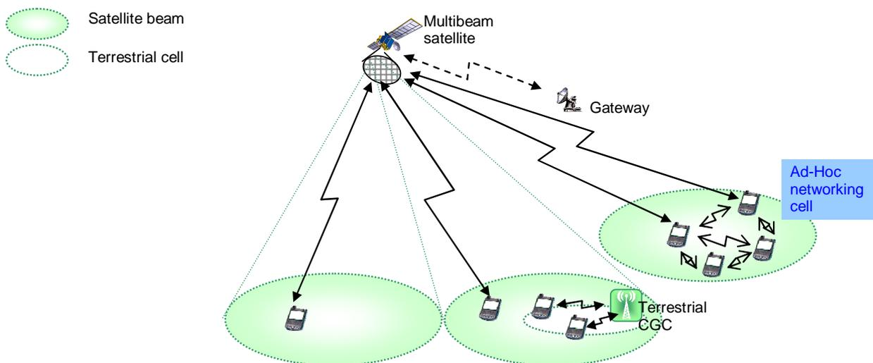
**Figure 7.6: System architecture with Ad-hoc networking capability**
