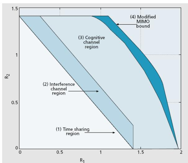
**Figure K.3: Rate regions ( $R_1$ ,  $R_2$ ) for different two-sender, two-receiver wireless channels**
