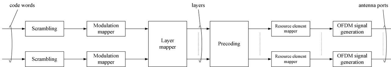
**Figure H.14: Overview of physical channel processing**
