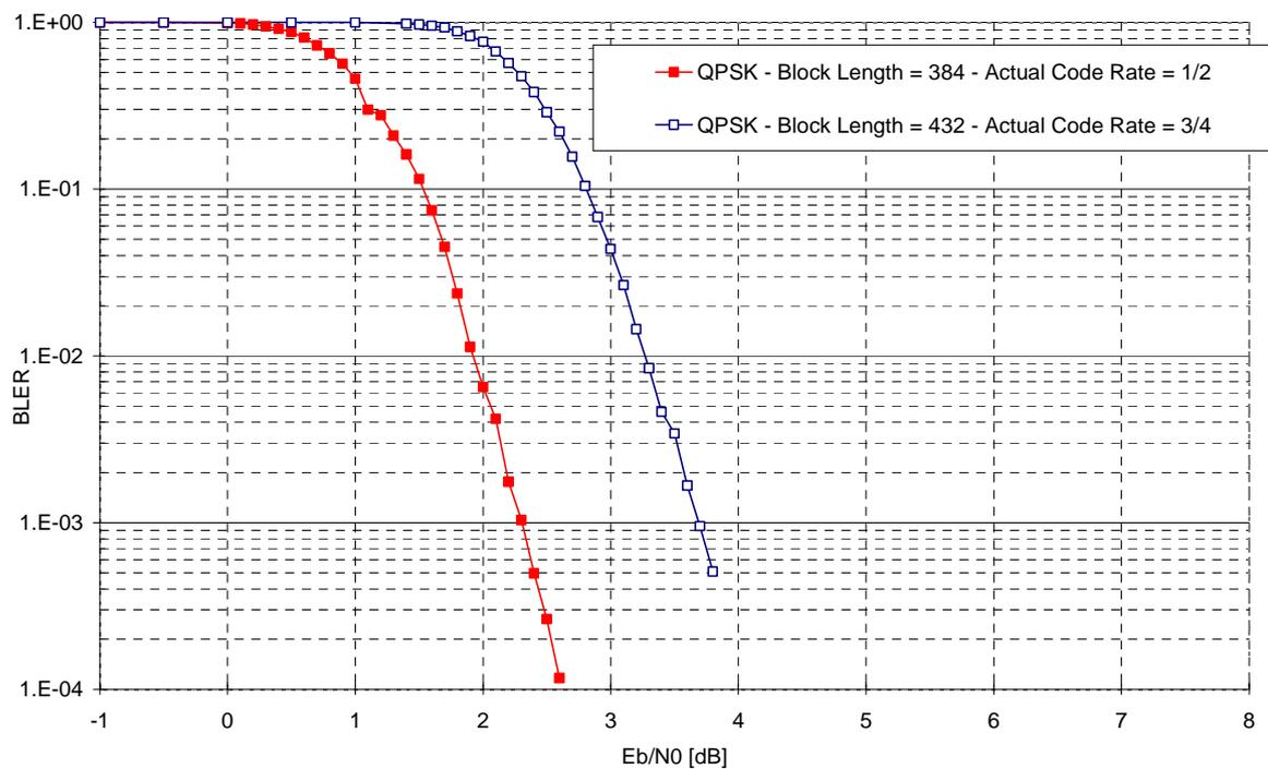
Figure I.29: BLER vs. Eb/N0 [dB], WiMAX Two-Way RL PHY configurations - Ideal Channel
