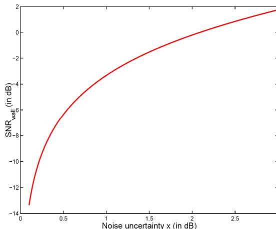
**Figure J.3: SNR Wall in Energy Detection Methods as Function of Noisy Power Uncertainty**
