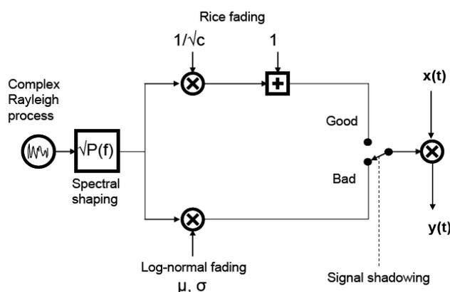
Figure A.3: Lutz two-state simulation model
