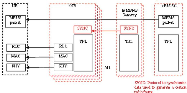
Figure H.10: The overall U-plane architecture of the MBMS content synchronisation
