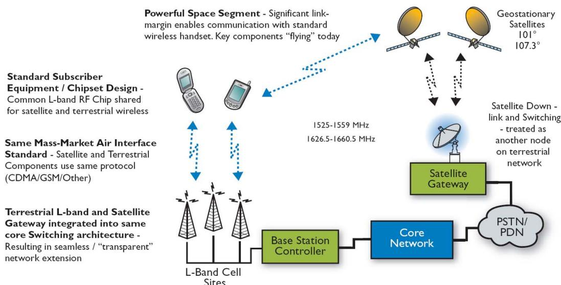
**Figure 6.3: Hybrid Terrestrial/Satellite Wireless Network**
