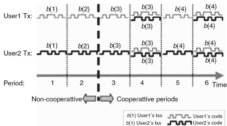
**Figure L.5: Practical Cooperative Scheme for CDMA Systems Proposed in [i.229] to [i.243]**
