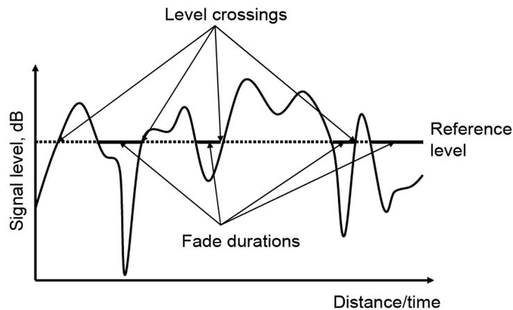
**Figure A.2: Level crossing and fade duration**
