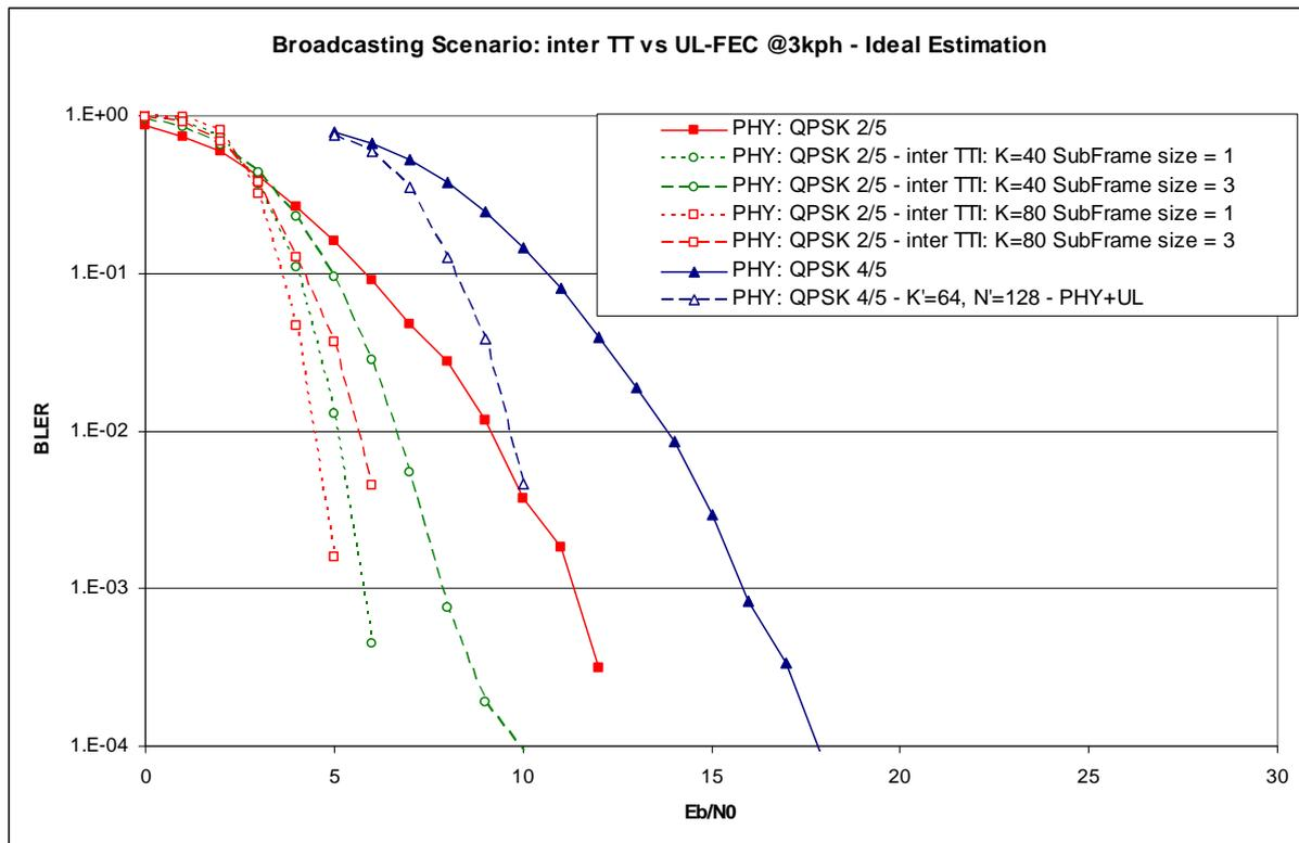
Figure I.44: Comparison between UL-FEC and interTTI. BLER vs Eb/N0
