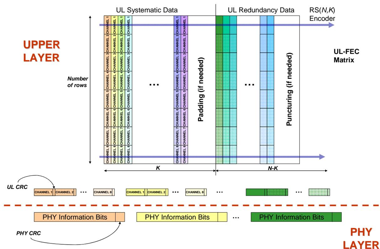
**Figure I.34: Block Diagram of the proposed Upper Layer FEC technique (Transmitter side)**
