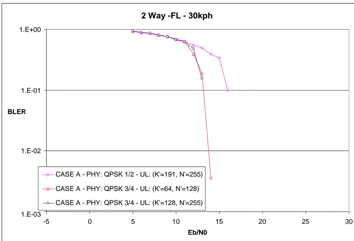
**Figure I.42: BLER performance obtained by splitting the redundancy between physical layer and upper layer keeping the total spectral efficiency. 2Way FL - 30 kph**
