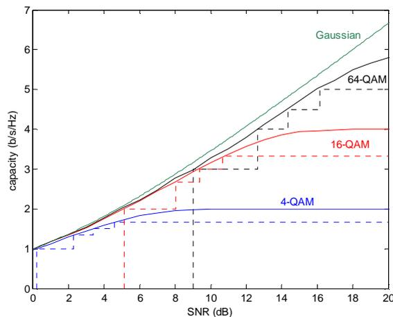
**Figure I.60: SNR-to-rate mapping**
