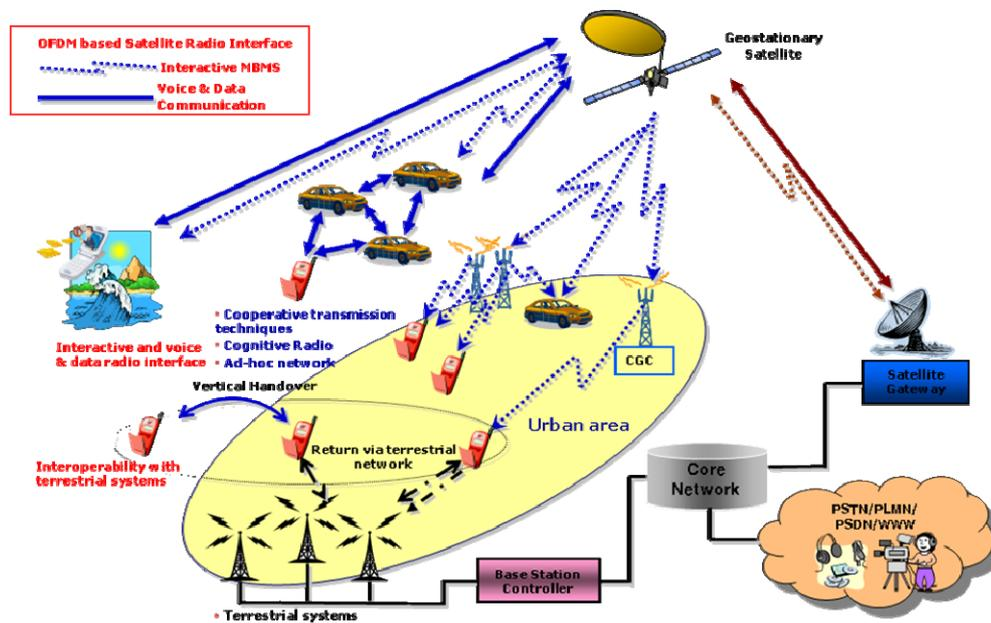
Figure 7.7: Hybrid satellite and terrestrial system architecture
