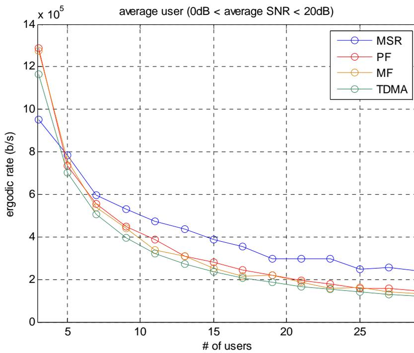
Figure I.50: average user rate performance (1,25 MHz system)
