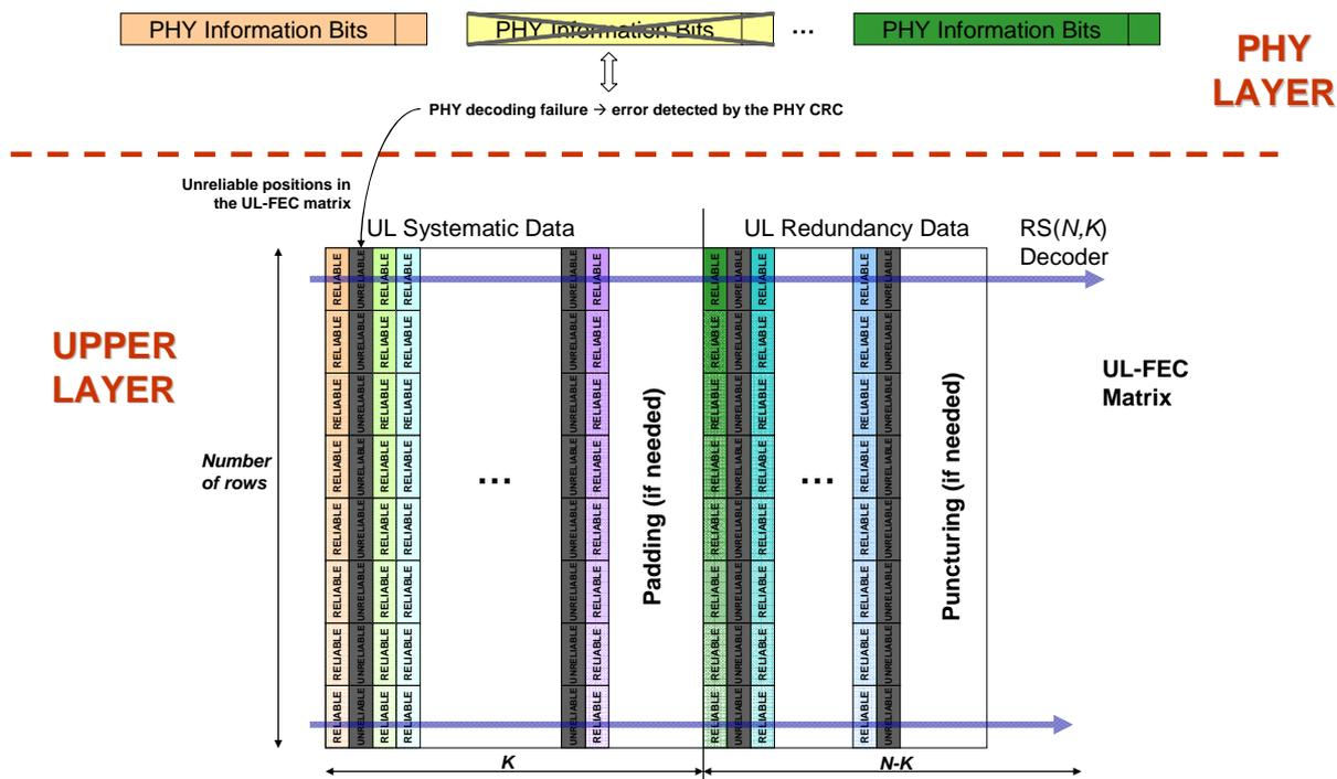
Figure I.35: Block Diagram of the receiver when CASE A is considered
