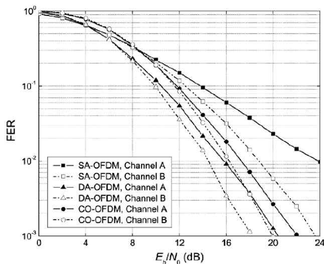
Figure L.9: The overall FER performance of the CO-OFDM system
