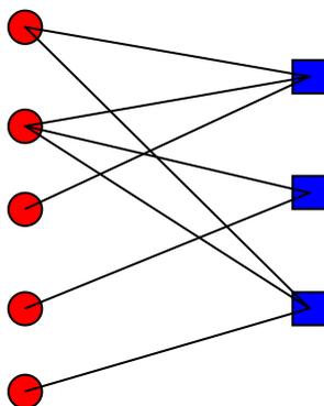
Figure E.3: Graph of the code described by equation (E.3)
