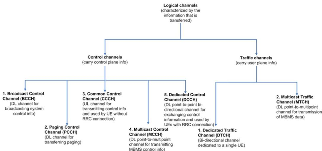
Figure H.6: Logical Channels in LTE
