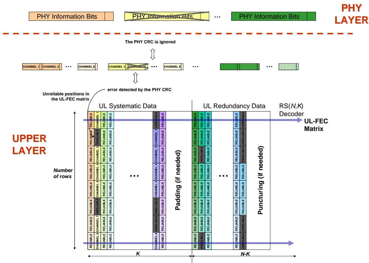
Figure I.36: Block Diagram of the receiver when CASE B is considered
