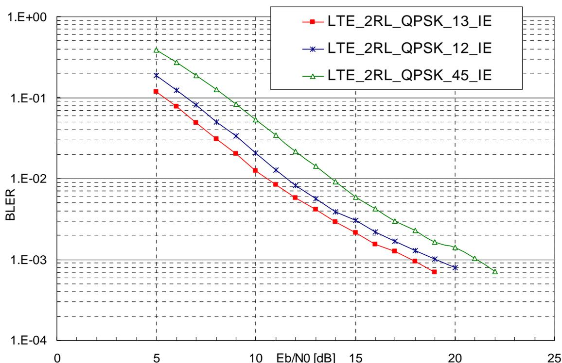
Figure I.30: BLER vs.  $E_b/N_0$  [dB], LTE Two-Way RL PHY configurations - Ideal Estimation
