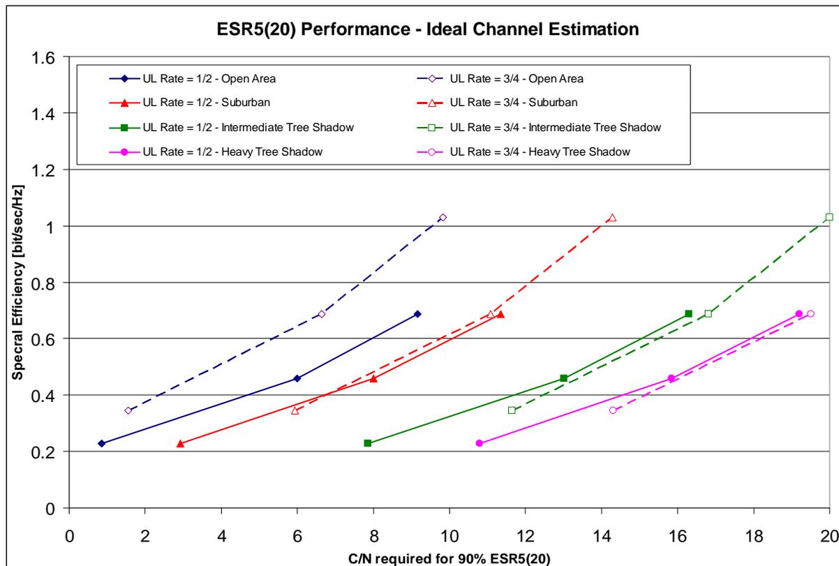
Figure I.46: Overall (PHY+UL) Spectral Efficiency vs C/N for 90 % ESR5(20)
