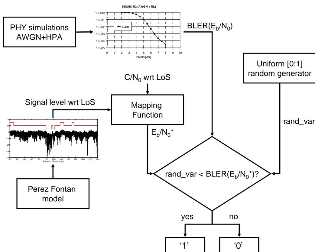
**Figure I.3: Block diagram of the procedure adopted for generating the time series**
