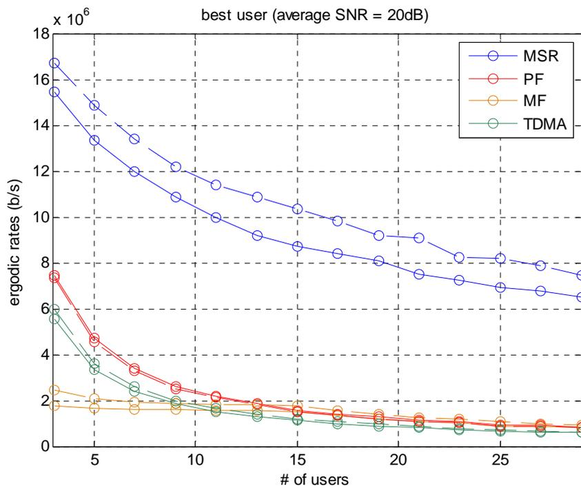
Figure I.53: best user rate performance (5 MHz system). Solid lines: (1, 1), Dashed lines: (2, 1)
