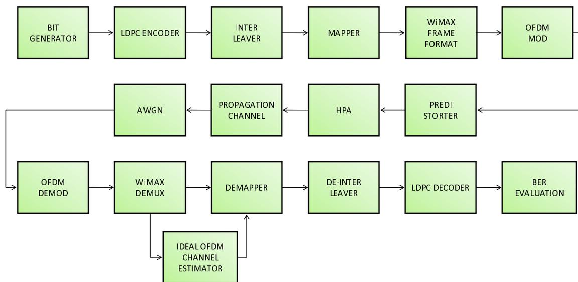
Figure I.2: WiMAX FL & RL - Ideal estimation simulation block diagram
