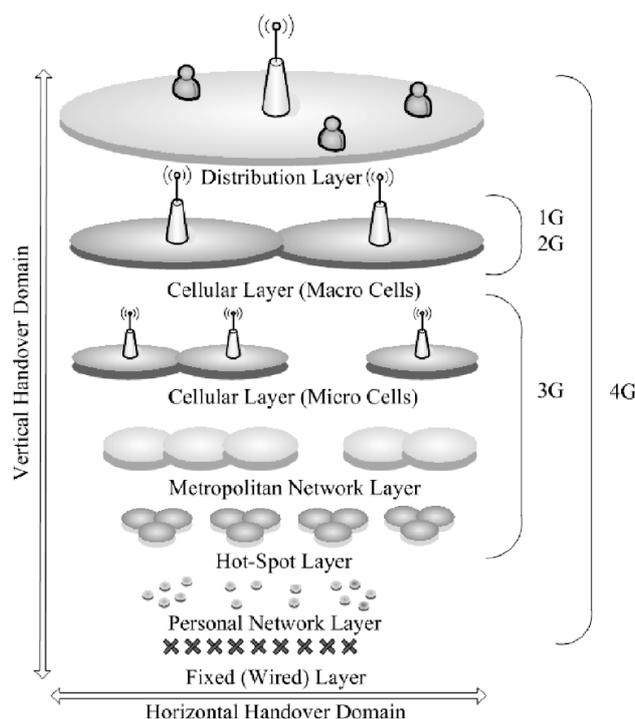
**Figure 6.1: Network-Level Architecture in 4G**
