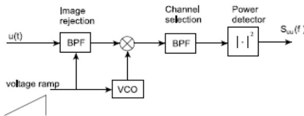
**Figure J.1: Scan-Based Super-Heterodyne Energy-Detection Architecture**
