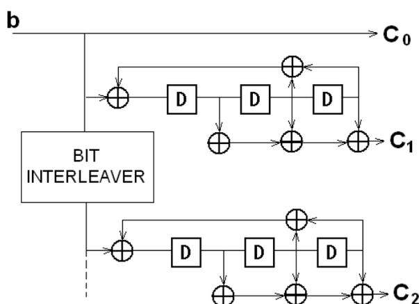
Figure E.1: Rate 1/3 Parallel Concatenated Systematic Turbo Code
