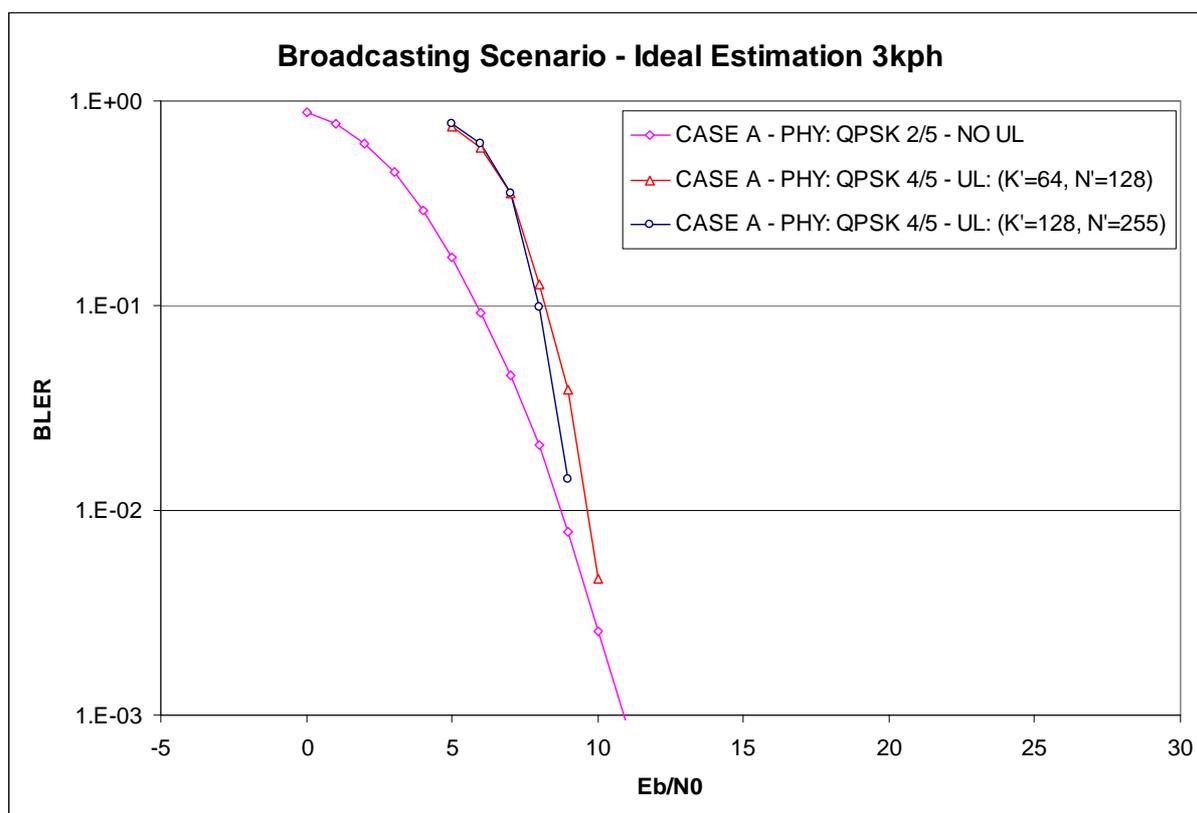
**Figure I.40: BLER performance obtained by splitting the redundancy between physical layer and upper layer keeping the total spectral efficiency. Broadcasting Scenario - Ideal Estimation - 3 kph**
