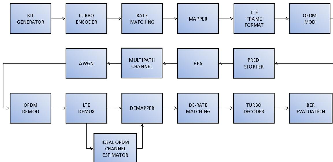
Figure I.1: LTE - Ideal estimation simulation block diagram
