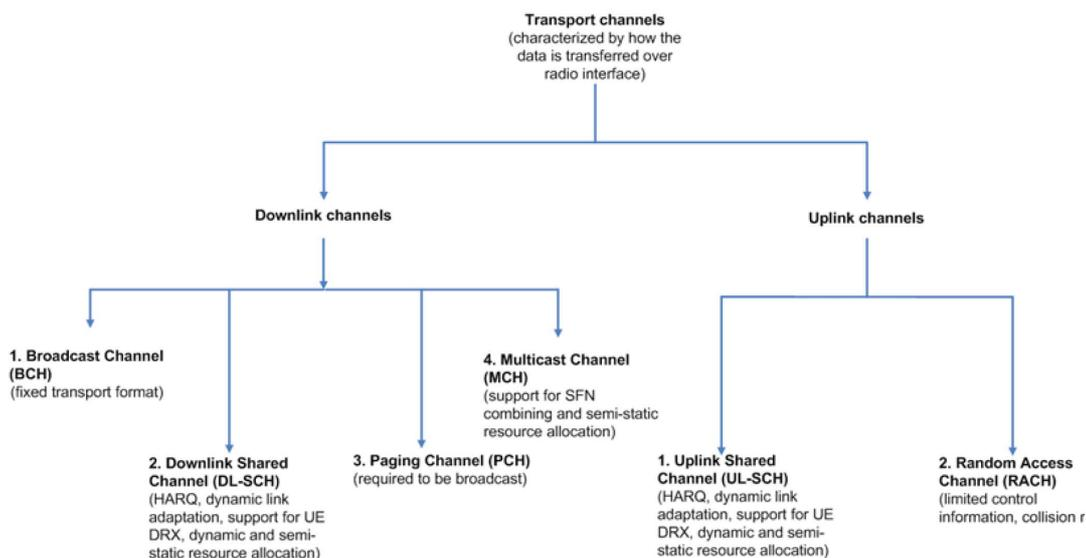
Figure H.7: Transport Channels in LTE
