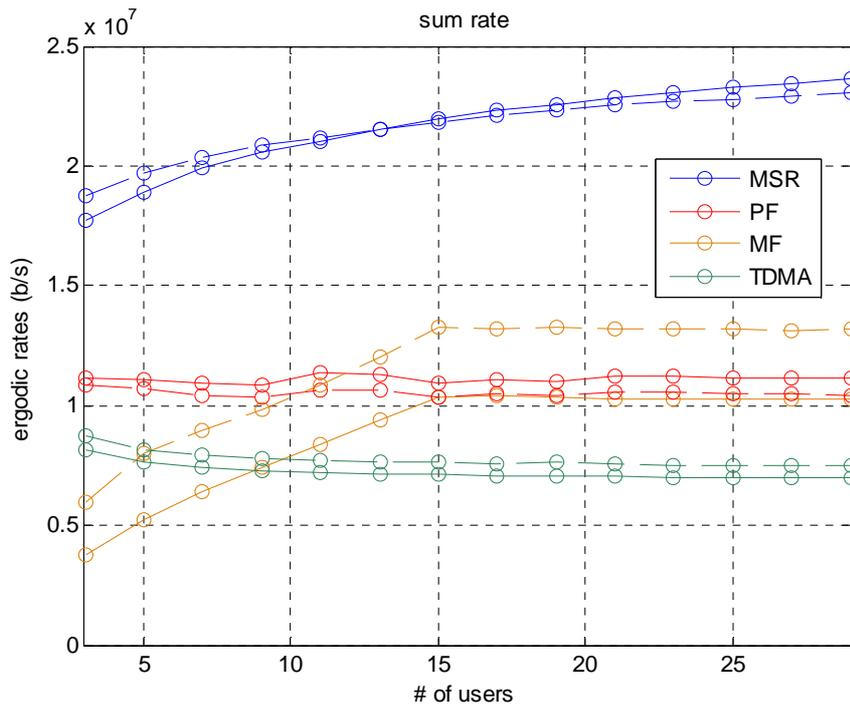
Figure I.52: Sum rate performance (5 MHz system). Solid lines: (1, 1), Dashed lines: (2, 1)
