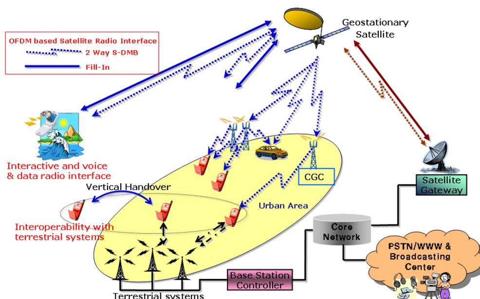
Figure N.1: Two potential services provided by IMT-Advanced satellite systems
