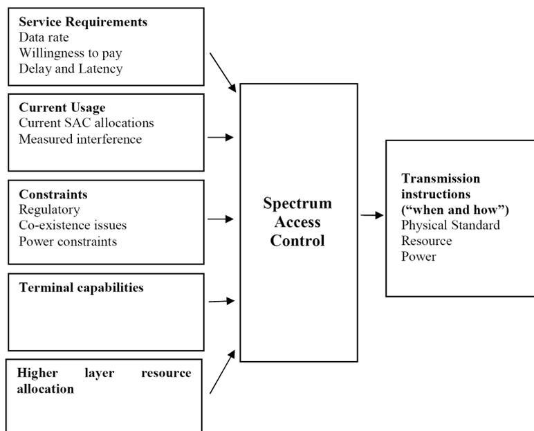
**Figure J.4: SAC Operation in Terms of Input Parameters and Action Decisions**
