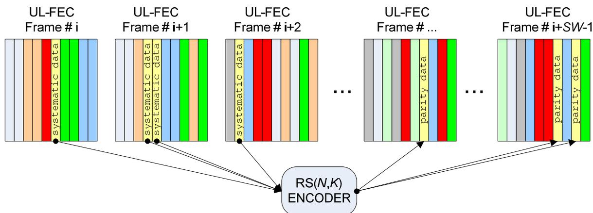
Figure I.39: UL-FEC with Sliding Window
