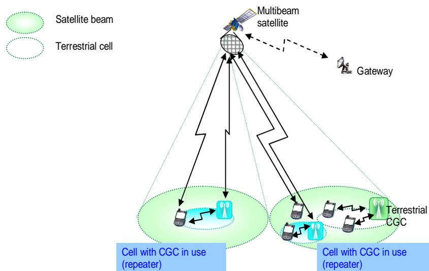
**Figure 7.4: System architecture with the use of complementary ground component (type2) used as a repeater**
