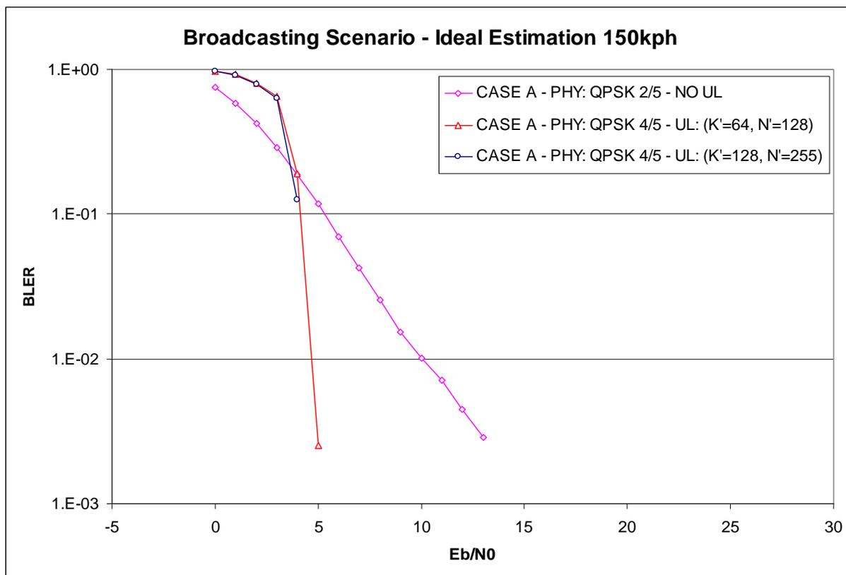
**Figure I.41: BLER performance obtained by splitting the redundancy between physical layer and upper layer keeping the total spectral efficiency. Broadcasting Scenario - Ideal Estimation - 150 kph**
