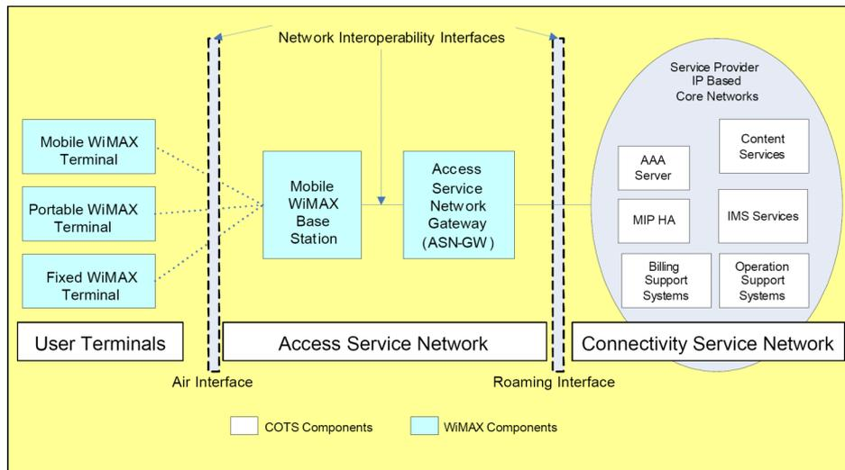
**Figure G.6: Overview of the Network IP-based architecture**
