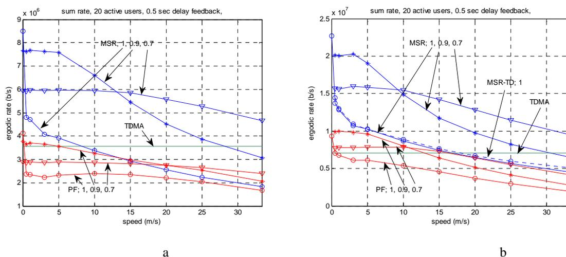
Figure I.56: sum rate performance, a) 1,25 MHz system, b) 5 MHz system
