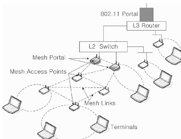
**Figure 6.6: The IEEE 802.11s mesh architecture**
