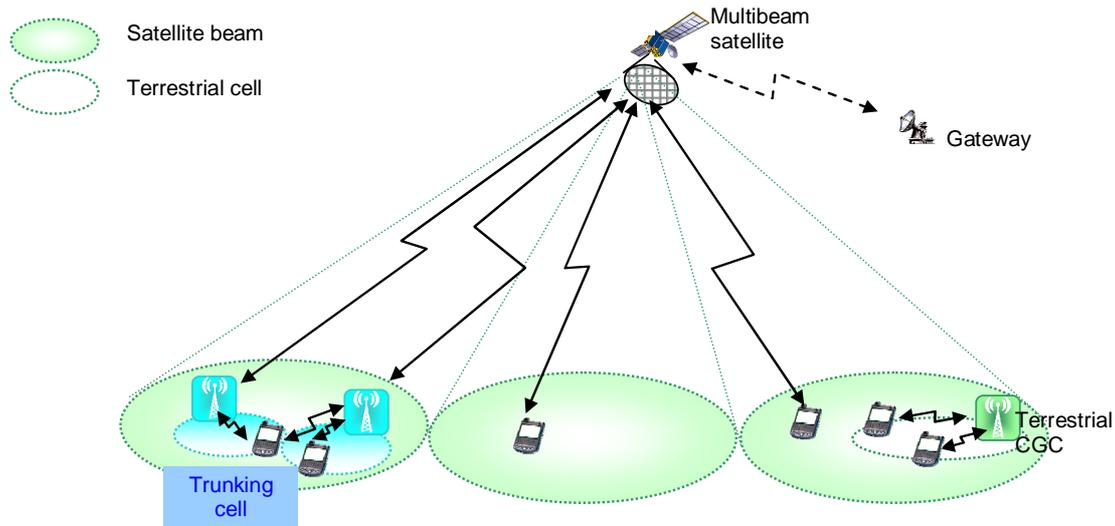
**Figure 7.5: System architecture with trunking capability**
