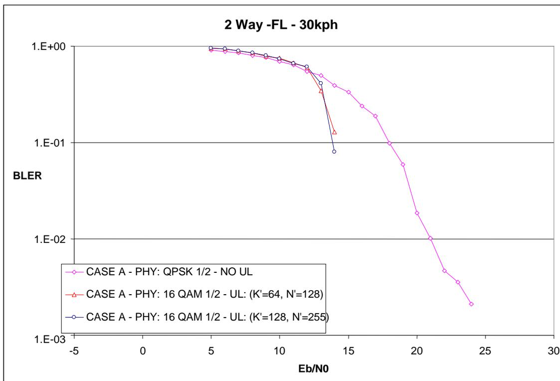
**Figure I.43: BLER performance obtained by splitting the redundancy between physical layer and upper layer keeping the total spectral efficiency. 2Way FL - 30 kph**
