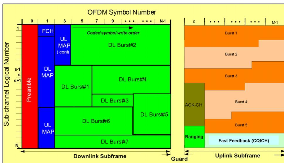
Figure G.1: WiMAX OFDM Frame Structure
