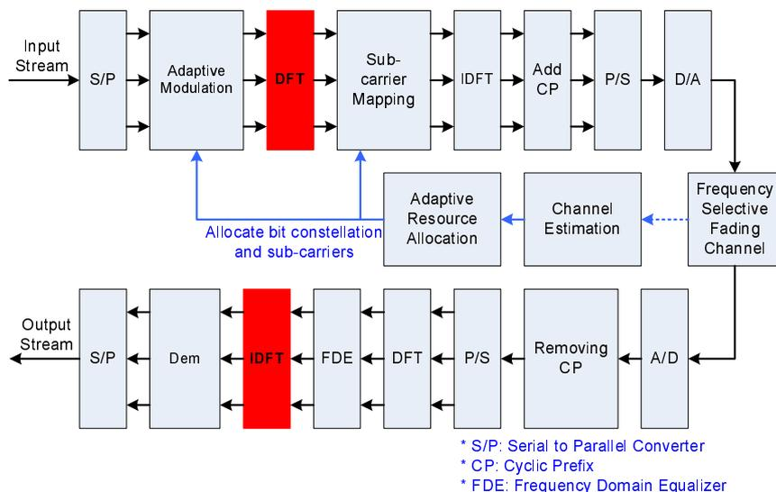
**Figure H.15: Block Diagram of Signal Processing functions in SC-FDMA**
