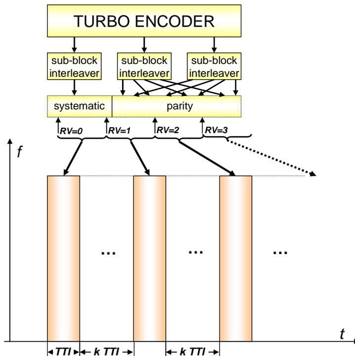
Figure I.5: Inter-TTI interleaving block diagram.
