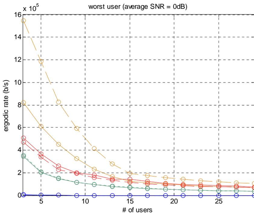
Figure I.55: worst user rate performance (5 MHz system). Solid lines: (1, 1), Dashed lines: (2, 1)
