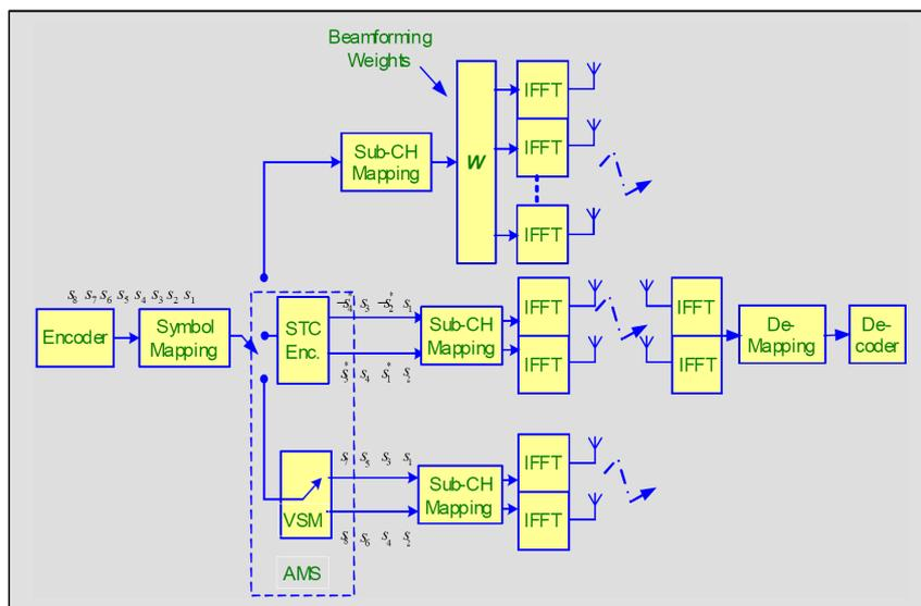
**Figure G.2: Adaptive MIMO switching**
