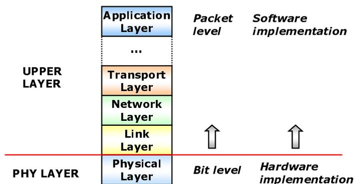
Figure I.32: Protocol stack and coding
