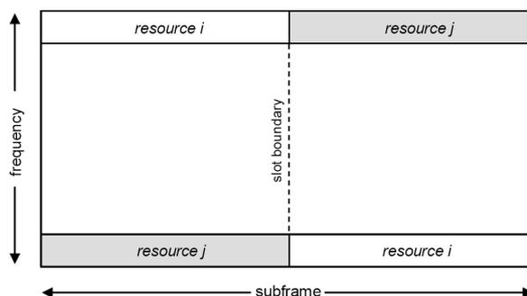
Figure H.16: PUCCH - hopped at slot boundary
