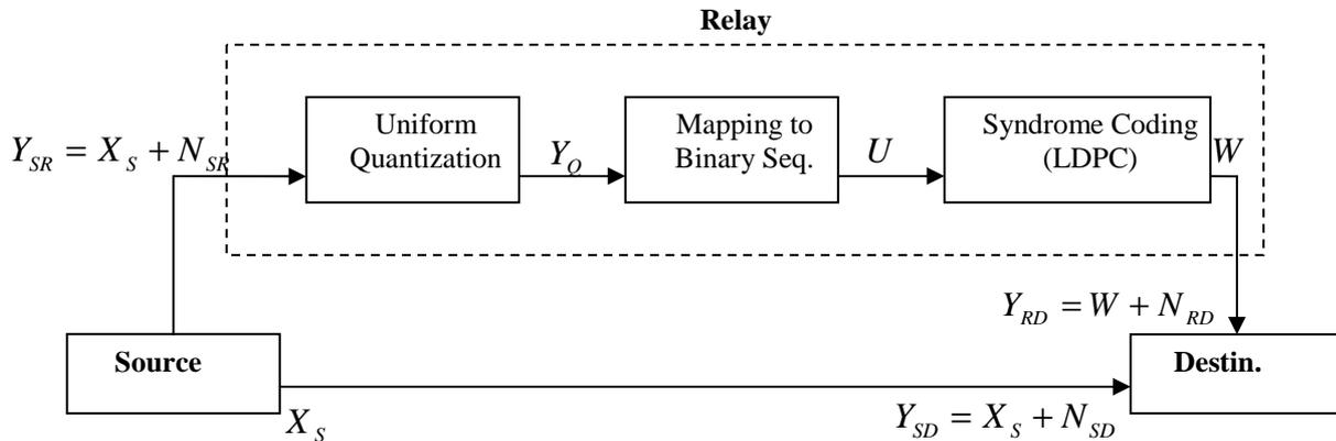
Figure L.2: Practical Compress and Forward Relay Model
