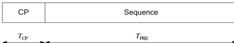
**Figure I.6: Random access preamble format**
