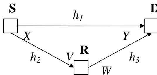
**Figure L-1: General Single Relay Channel**
