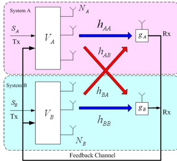
**Figure K.1: Block diagram of MISO Linear Precoded Co-existing Systems**
