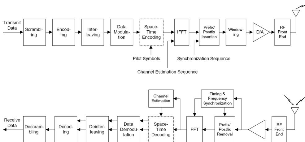
**Figure L.8: Block Diagram of the CO-OFDM Architecture proposed in [i.246] (dotted blocks are used only in the cooperation phase)**
