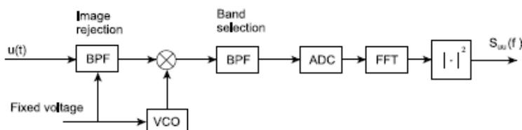
**Figure J.2: FFT-based Energy-Detection Architecture**
