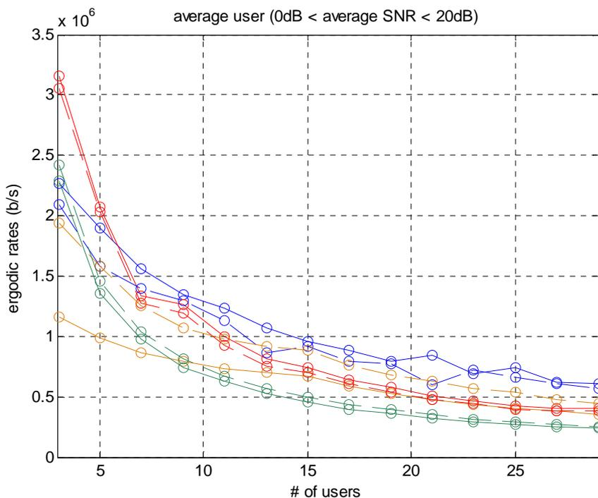
Figure I.54: average user rate performance (5 MHz system). Solid lines: (1, 1), Dashed lines: (2, 1)
