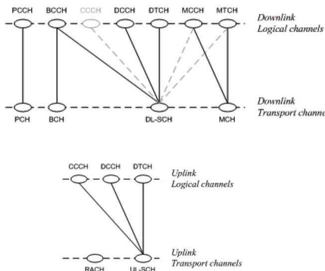
**Figure H.8: Logical to Transport channel mappings**
