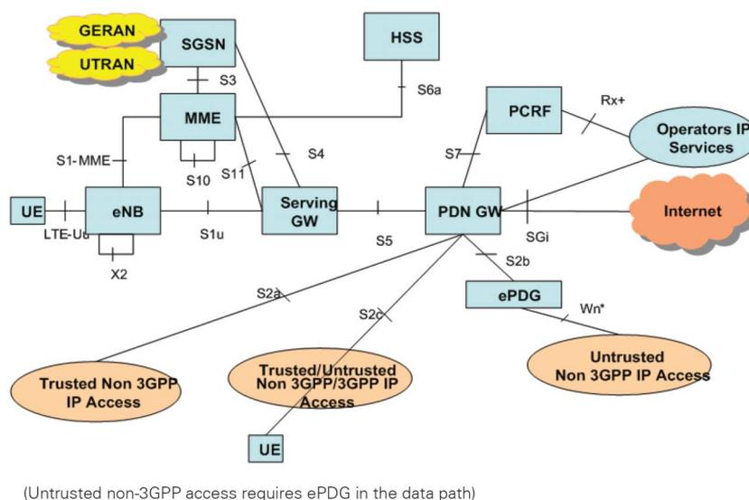
**Figure H.1: High-level architecture of 3GPP LTE**
