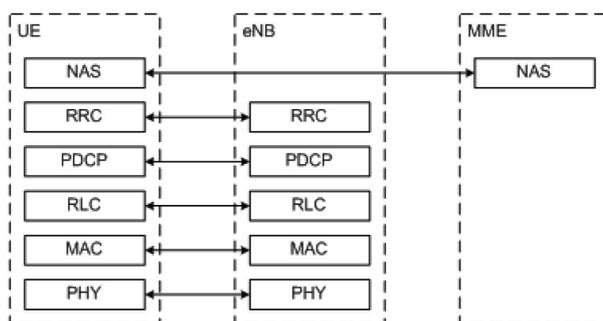
**Figure H.2: Control plane protocol stack**
