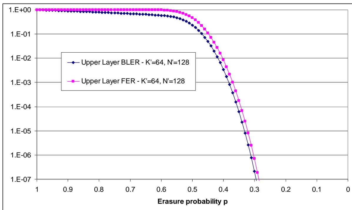
Figure I.38: Upper Layer BLER over the BEC. CASE A
