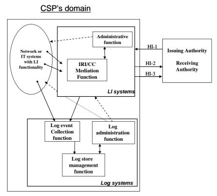
Figure 1: CSP functional architecture for the LI operation
