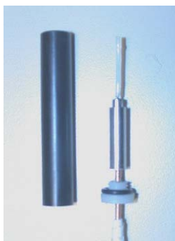
Figure B.4: Dipole without the cylindrical radome
