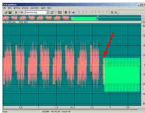
Figure 17: Combination of the Composite Source Signal in one transmission direction (red) and the uncorrelated voiced sound in the opposite direction (green) to switch between the two transmission directions
