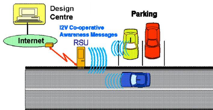
**Figure C.48: Vehicle data collection application scenario**
