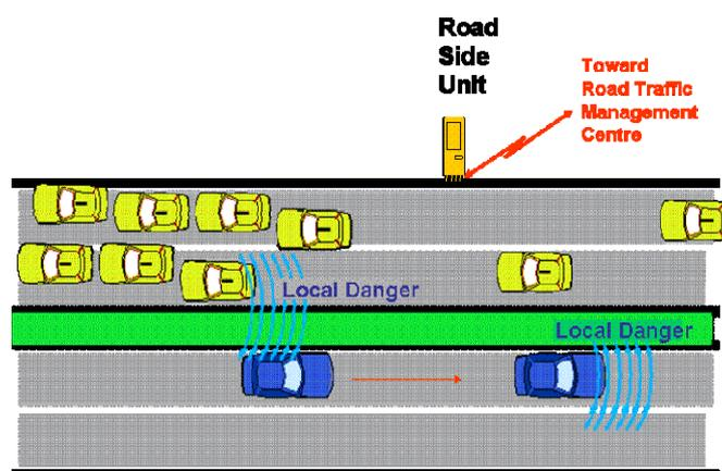
Figure C.12: Decentralized floating car data use case scenario
