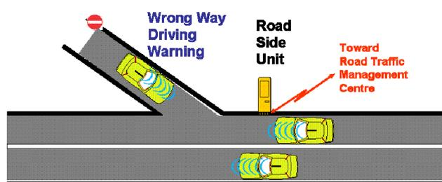
**Figure C.7: Wrong way driving warning use case scenario**
