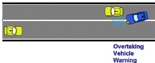
**Figure C.13: Overtaking vehicle warning use case scenario**
