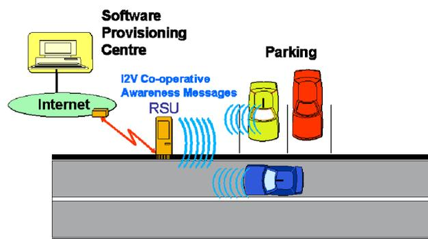
**Figure C.51: Vehicle software/data provisioning and update scenario**
