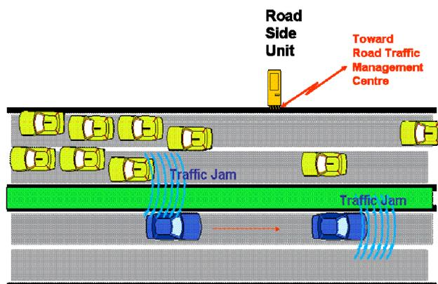
**Figure C.9: Traffic condition warning use case scenario**
