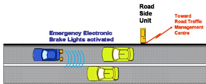
**Figure C.1: Emergency electronic brake lights use case scenario**
