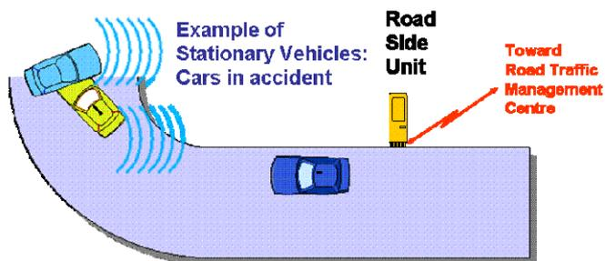
**Figure C.8: Stationary vehicle warning use case scenario**
