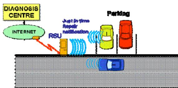
**Figure C.46: Remote diagnosis and just in time repair notification scenario**
