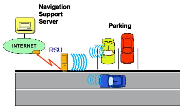
**Figure C.27: Enhanced route guidance and navigation use case scenario**
