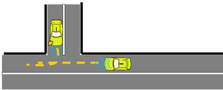
**Figure C.18: Merging traffic turn collision risk warning use case scenario**
