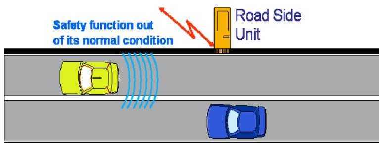
**Figure C.2: Safety function out of normal condition warning use case scenario**
