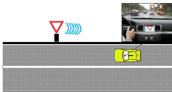
**Figure C.31: In vehicle signage use case scenario**
