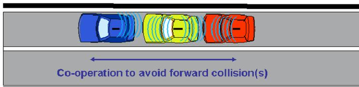
**Figure C.22: Co-operative forward collision warning use case scenario**
