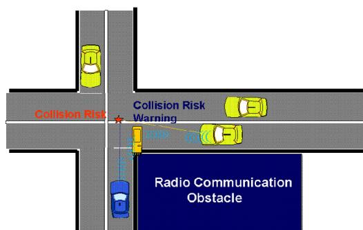
**Figure C.23: Collision Risk Warning from RSU use case scenario**
