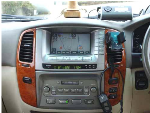
Figure A.24: Standard-fit MW/LW (AM) and Band II (FM) receiver in a Toyota Amazon The Pure Highway DAB receiver is also visible to the top right of the image
