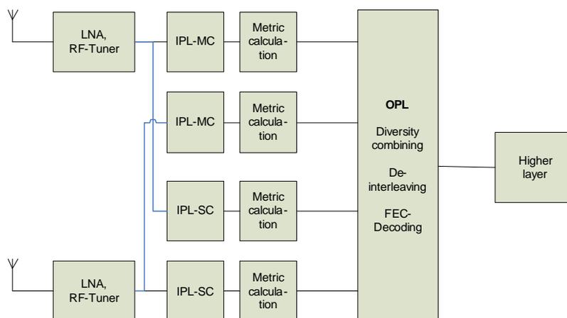
Figure 7.7: Hybrid receiver (single and multi-carrier) with antenna diversity
