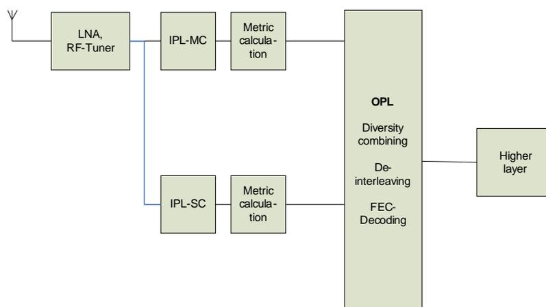
Figure 7.6: Hybrid receiver (single and multi-carrier) with only one antenna
