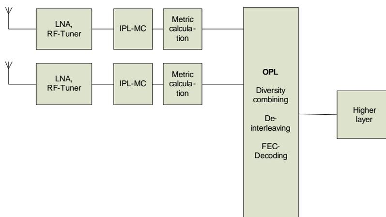
**Figure 7.4: Multi-carrier only receiver with two distinct antennas, maximum ratio combining**
