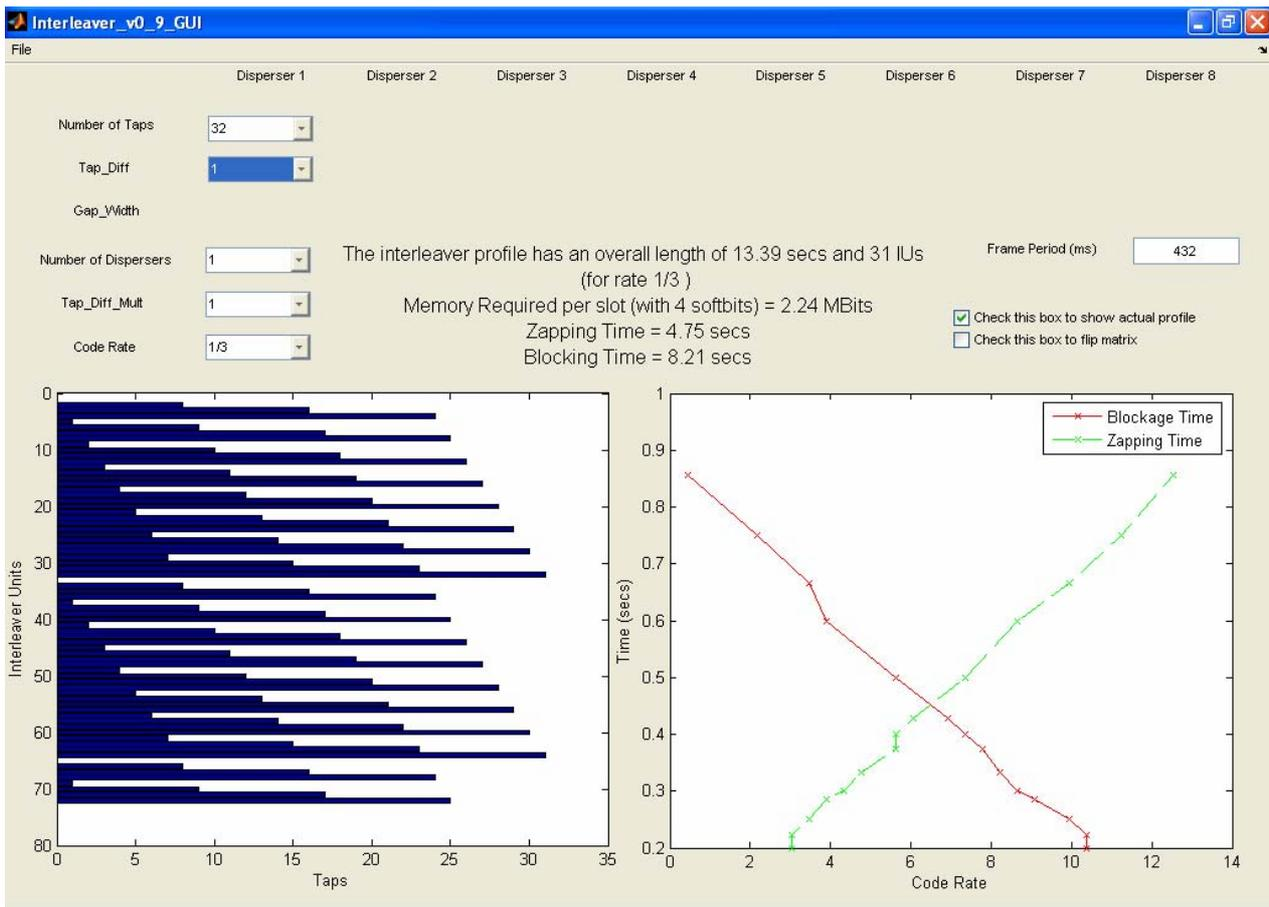
Figure 4.7: Example of uniform interleaver profile
