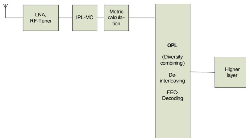
**Figure 7.2: Low cost receiver architecture**
