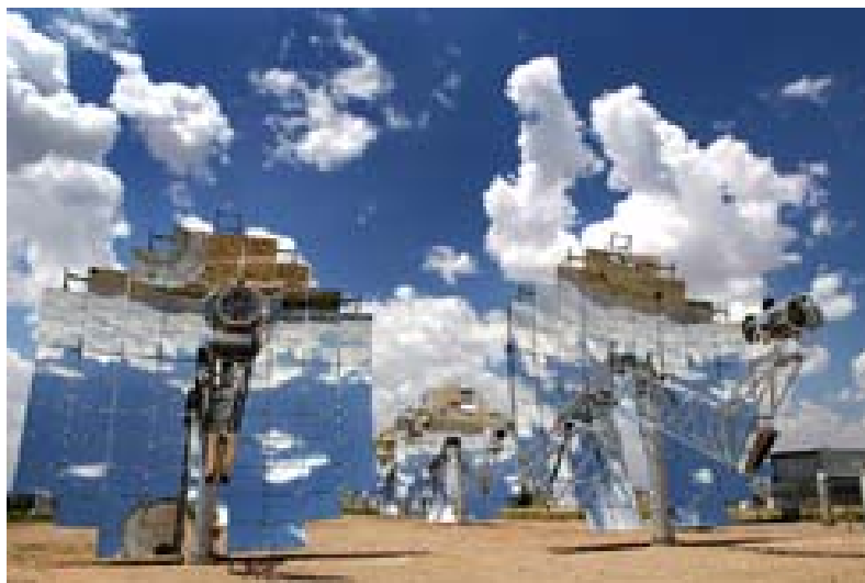
Figure 6: Stirling machine heated by sun concentrator (Sandia labs 2008)
