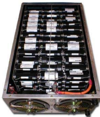
Figure 13: Supercapacitor Bank, 360 V -150 kW 320 WHr
