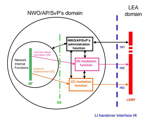
Figure 6: Functional block diagram showing Handover Interface HI
