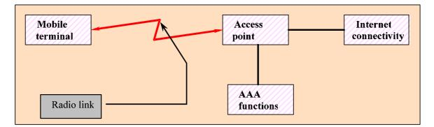
Figure 1: The elements of an IEEE 802.11 Internet access arrangement
