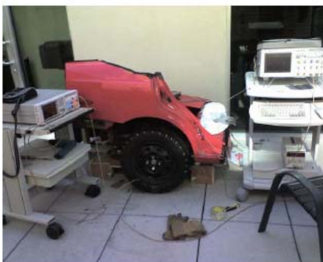
Figure B.15: Smart tire measurement set-up
