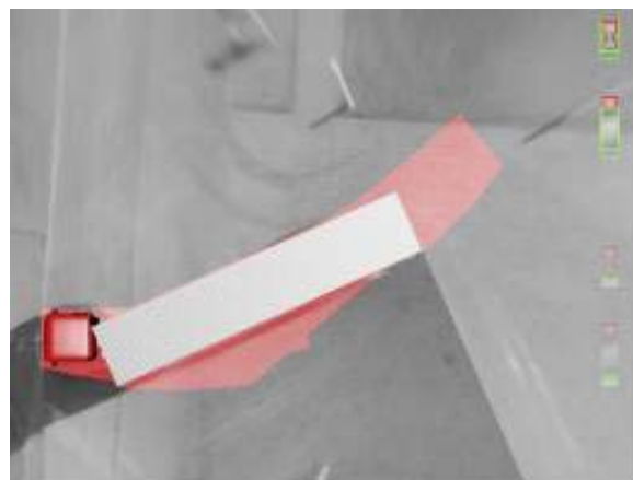
Figure B.10: The bird's-eye-view image shows the whole surrounding area of a truck-trailer combination
