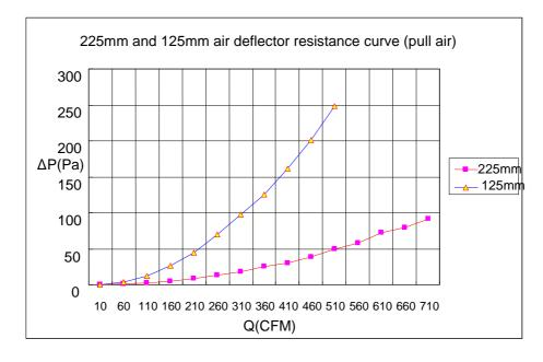
Figure A.3.4.2b: Test data of pull air pressure loss of deflector
