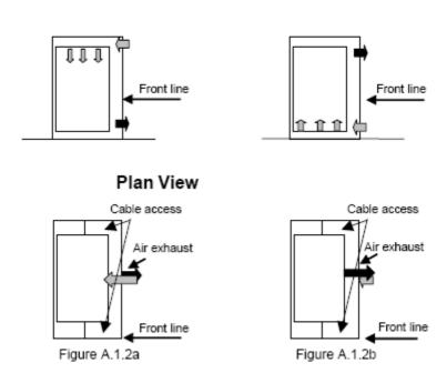
Either of the above configurations can be placed on a raised floor. The configuration in figure A.1.2b can also use an air inlet in the bottom of the ARCM.
