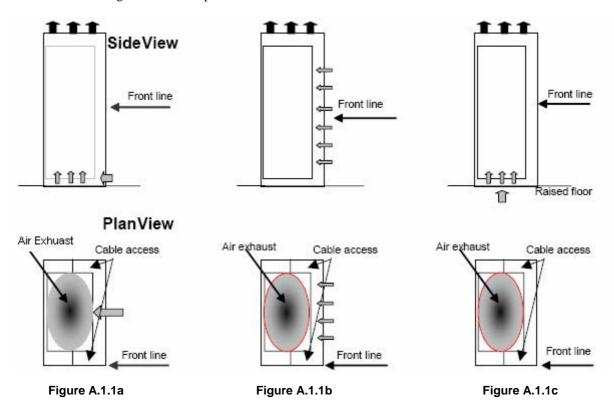
Combinations of the air inlet configurations shown above have also been used. Any of the above configurations could also have an air inlet in the bottom of the ARCM.
