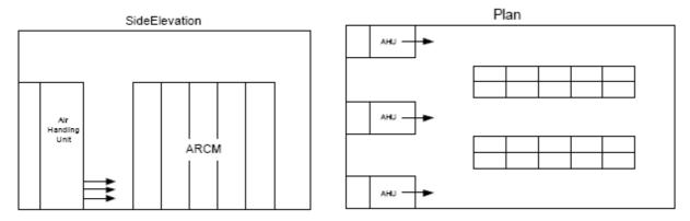
Figure 6.3.2.4b: Option B Free Blow along the aisles
