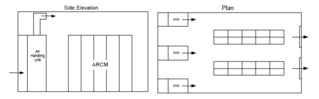
Figure 6.3.2.4a: Option A Free blow at high level
