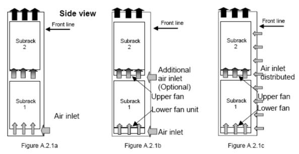
Any of the above configurations could also have an air inlet in the bottom of the ARCM.
