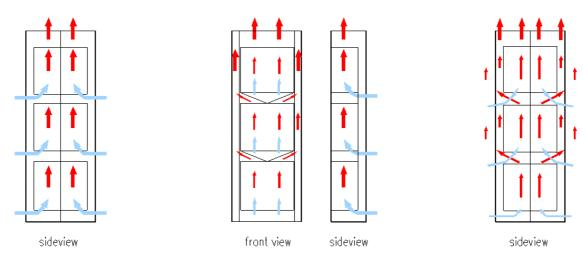
Figure B.3.1: ETSI 300 mm ARCM solution
