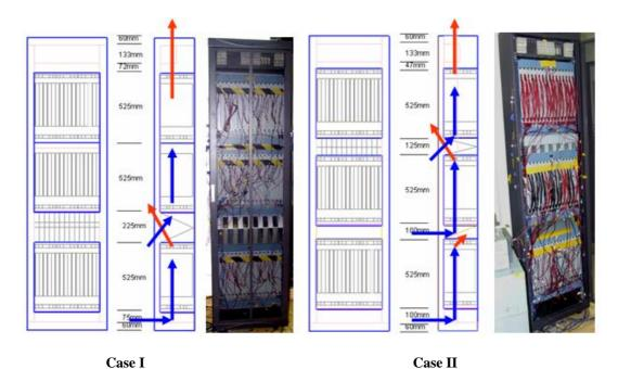
Figure A.3.4.2a: Test configuration for different size air deflector
