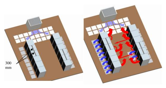
Figure B.3.2a: 300 mm cabinet in same line with 600 mm cabinet in central office
