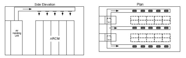
Figure 6.3.2.4d: Option B Overhead Distribution via a network of ducts
