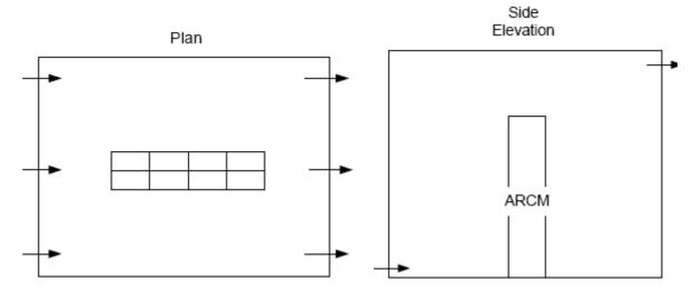
Figure 6.3.2.1a: Option A Passive Cooling
