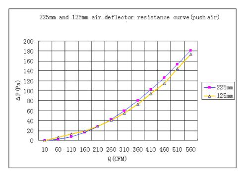
Figure A.3.4.2c: Test data of push air pressure loss of deflector
