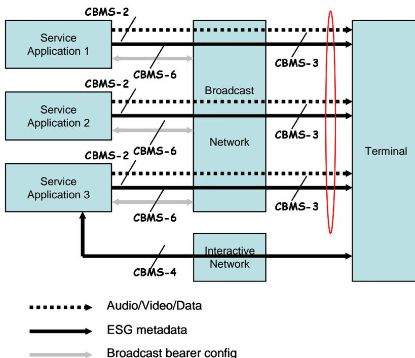
**Figure 5: Distributed ESG provisioning**
