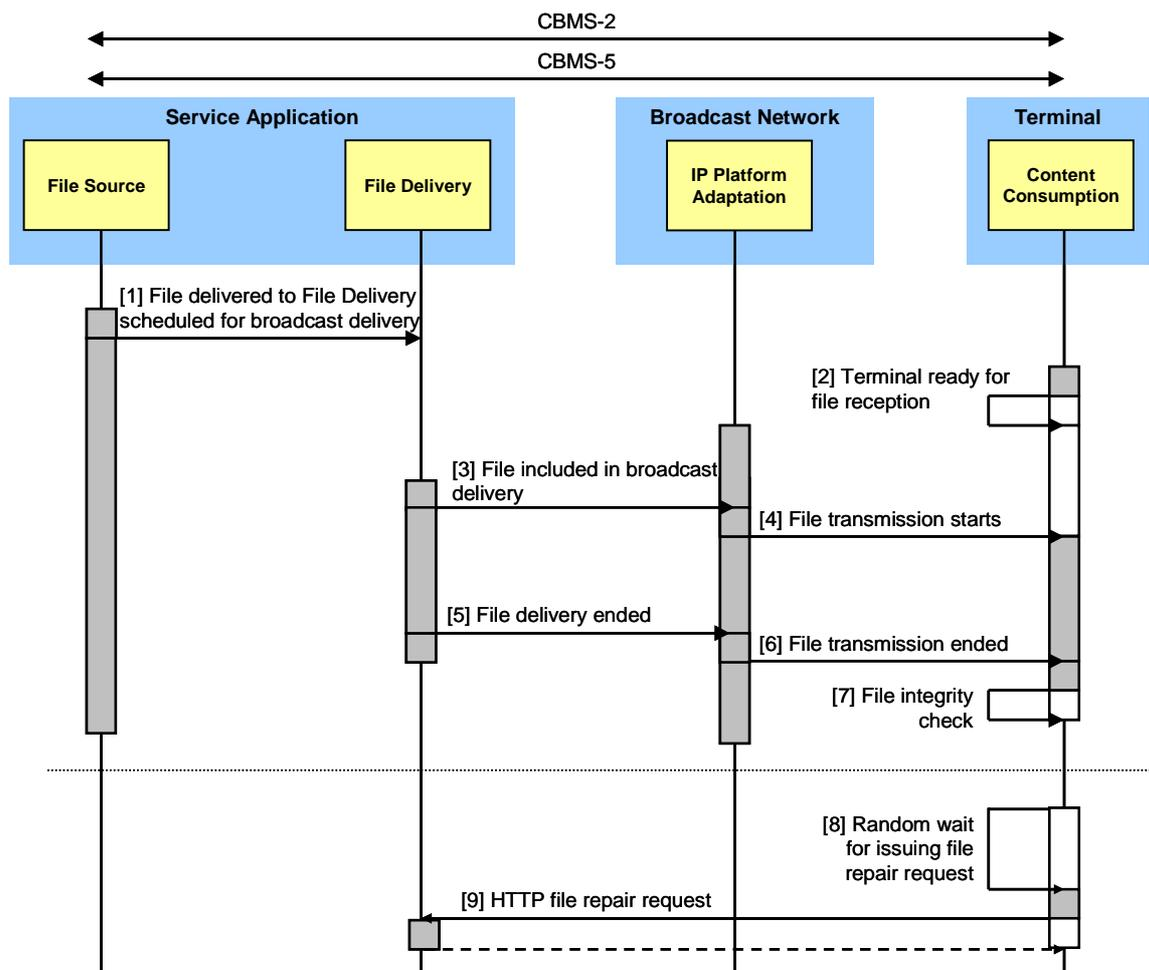
**Figure 12: Message flow for File Delivery**
