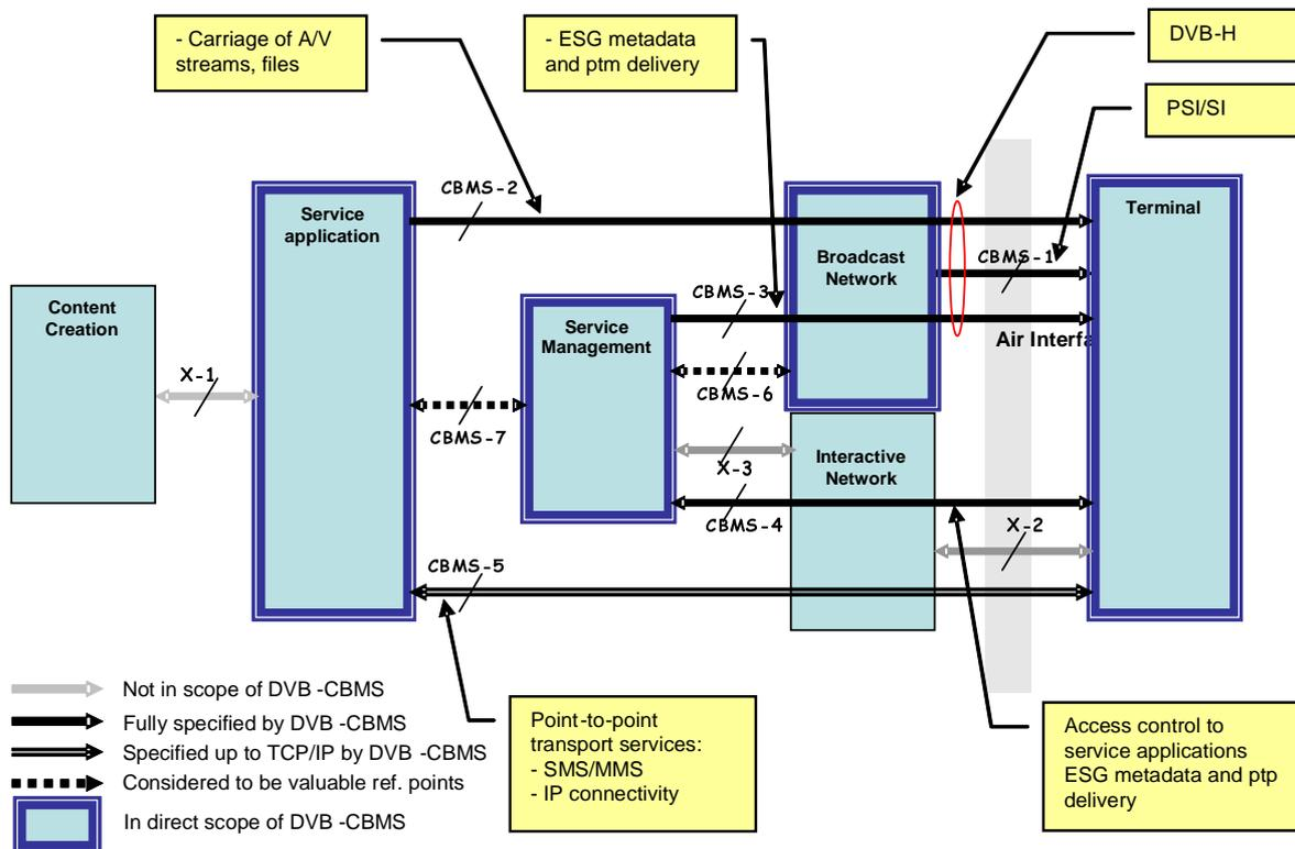
Figure 1: Proposed Architecture Diagram
