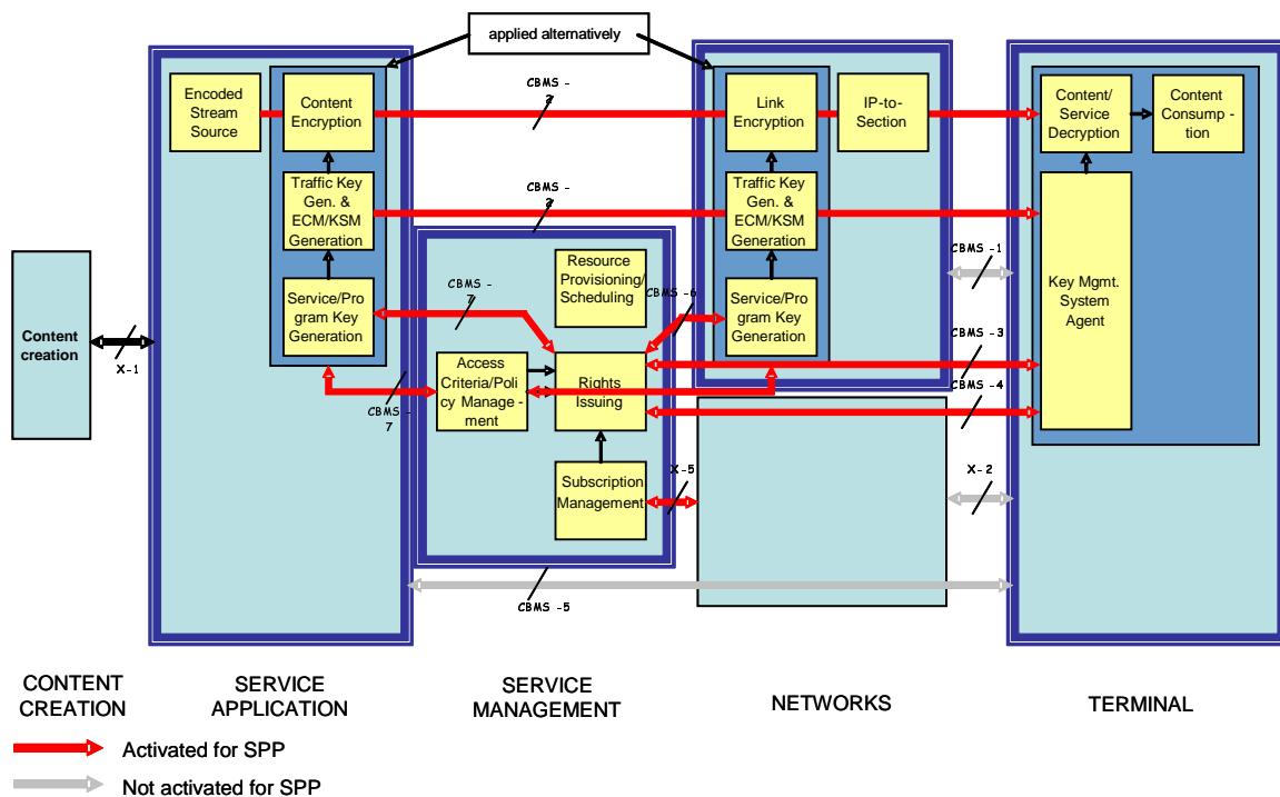
**Figure 14: Sub-Entities and reference points activated for Service Purchase and Protection**
