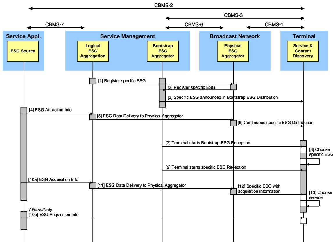
**Figure 8: Interactions for ESG provisioning**
