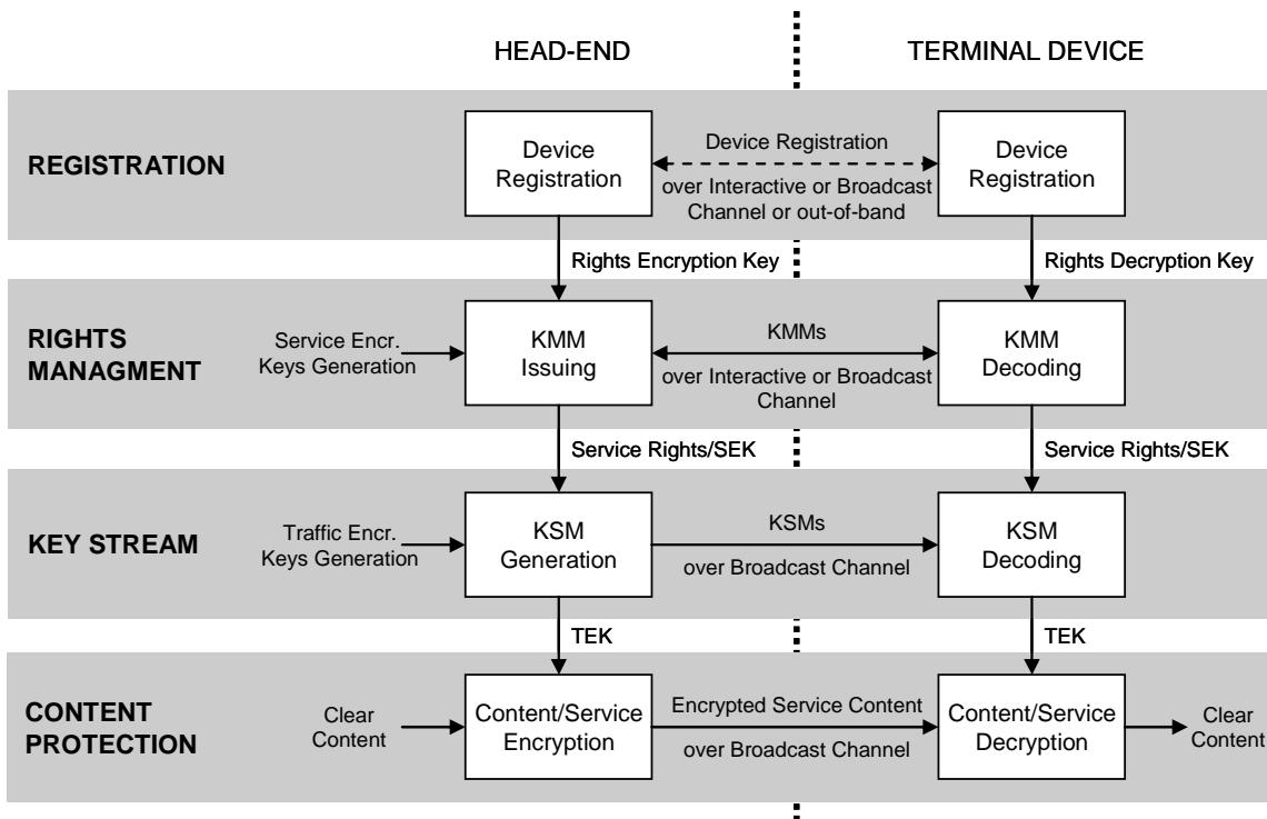
**Figure 13: Hierarchical Model for Service Protection**
