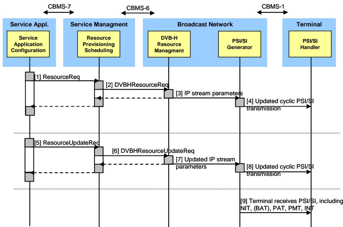
Figure 3: Message flow for service configuration
