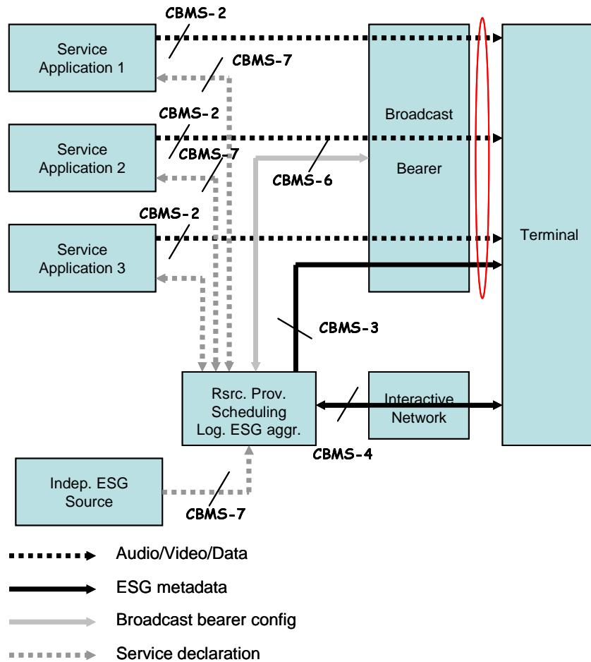
**Figure 6: Centralized ESG provisioning**
