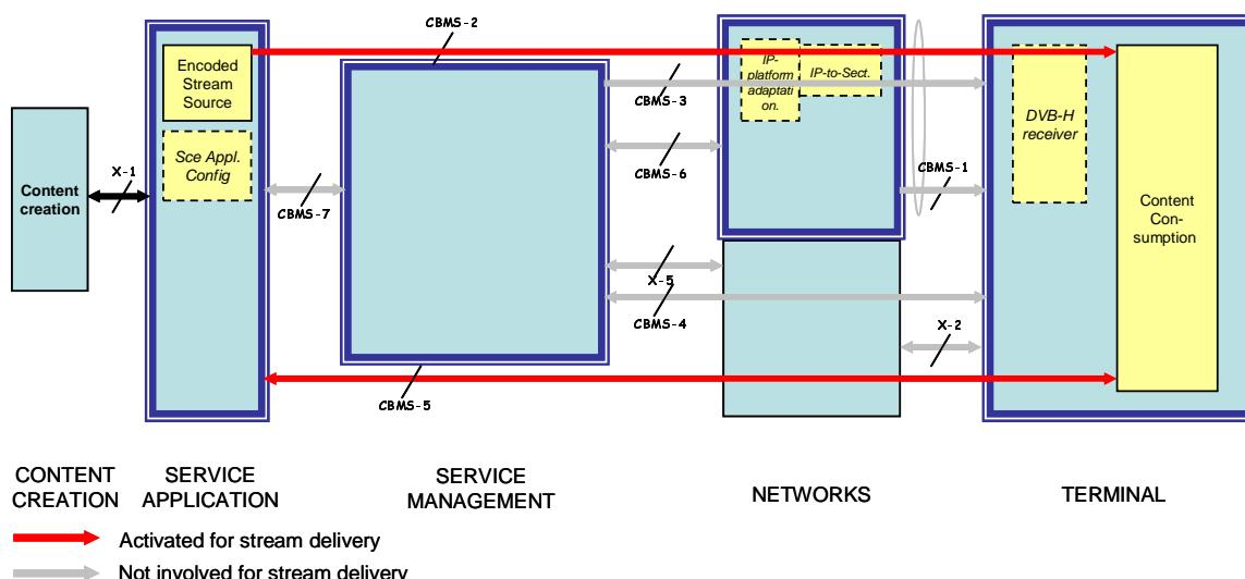
**Figure 9: Reference points activated for stream delivery**
