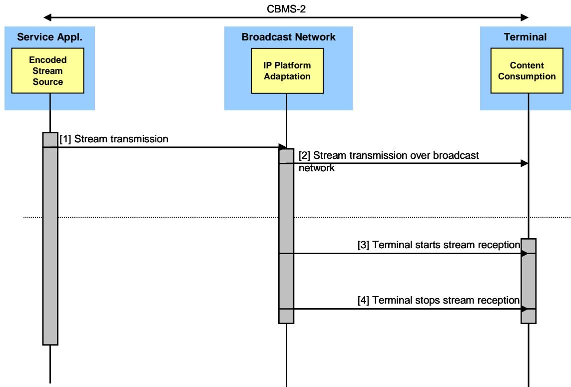
**Figure 10: Message flow for Stream Delivery**
