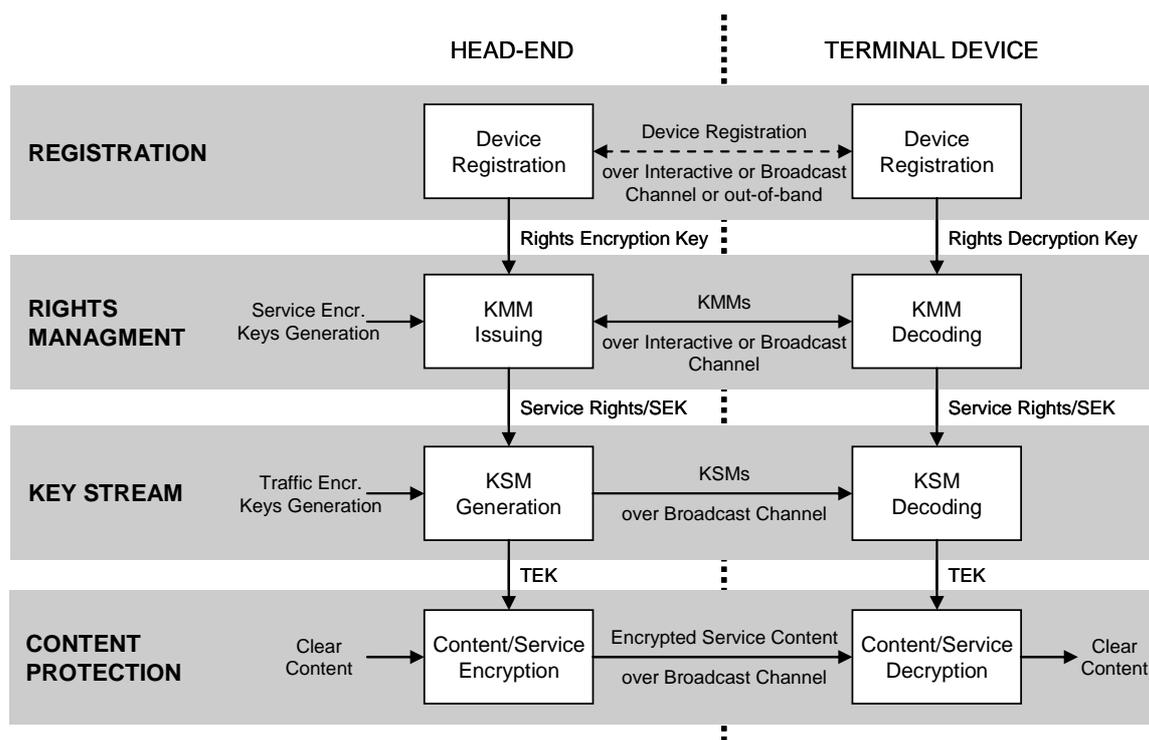
**Figure 13: Hierarchical Model for Service Protection**
