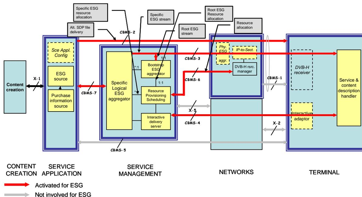
Figure 4: Reference points activated for ESG
