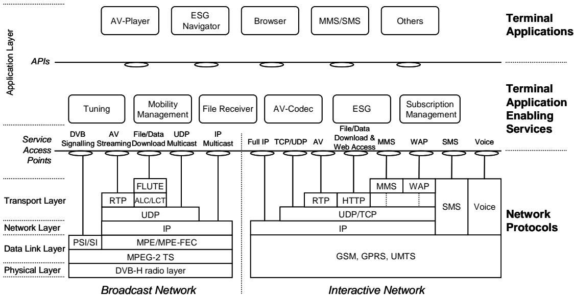
**Figure 16: Protocol, Enablers, Applications Hierarchy in IP Datacast**
