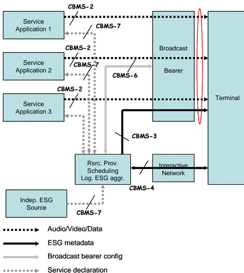
**Figure 6: Centralized ESG provisioning**
