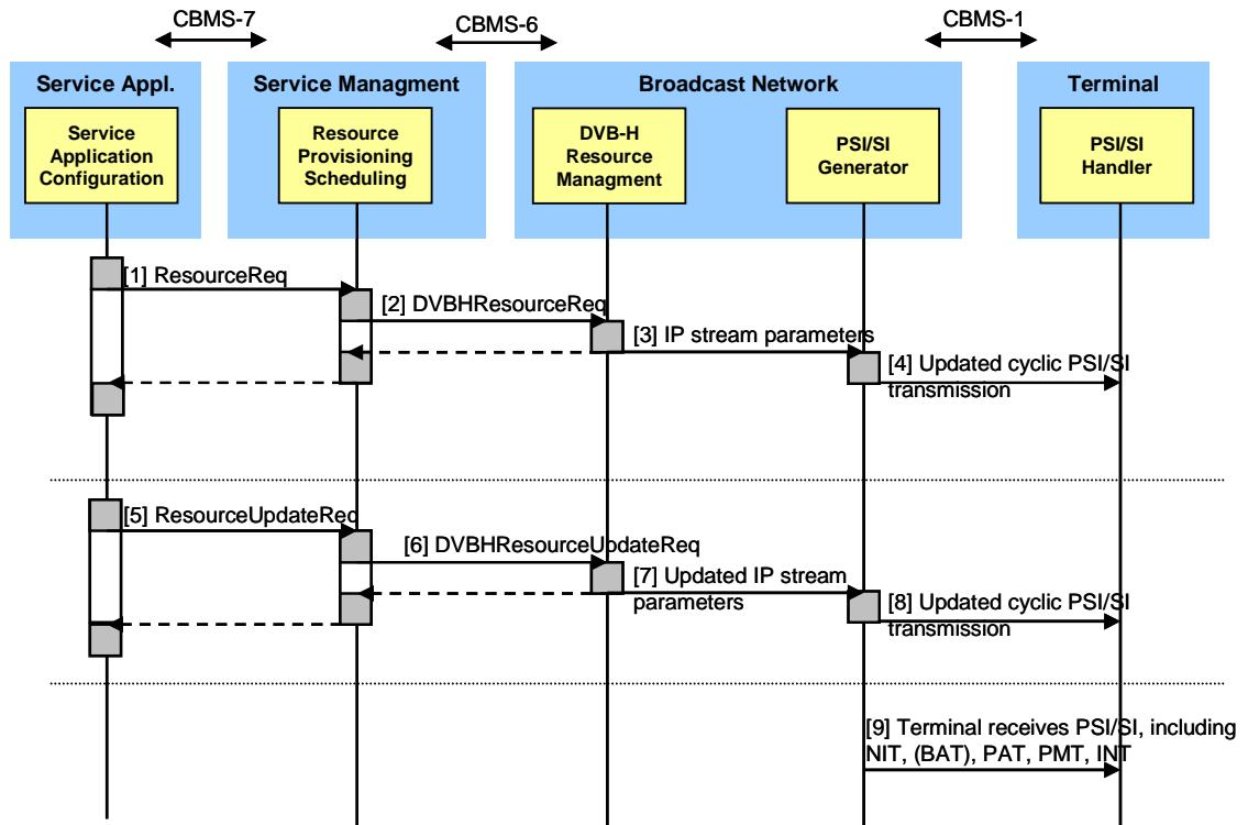
Figure 3: Message flow for service configuration
