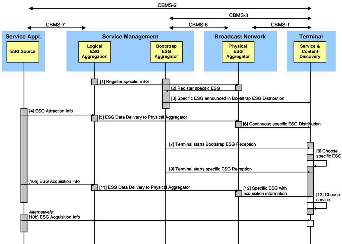
**Figure 8: Interactions for ESG provisioning**
