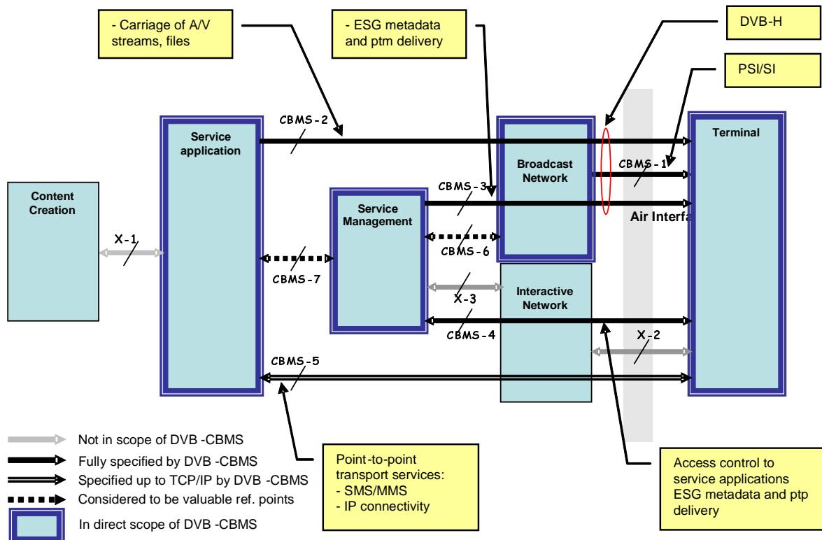
Figure 1: Proposed Architecture Diagram
