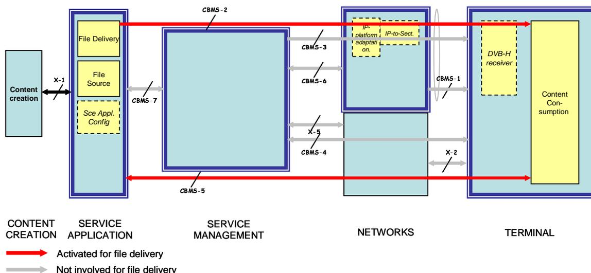
Figure 11: Reference points activated for file delivery
