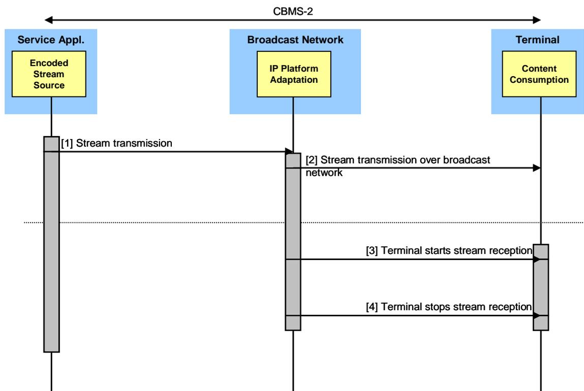
**Figure 10: Message flow for Stream Delivery**
