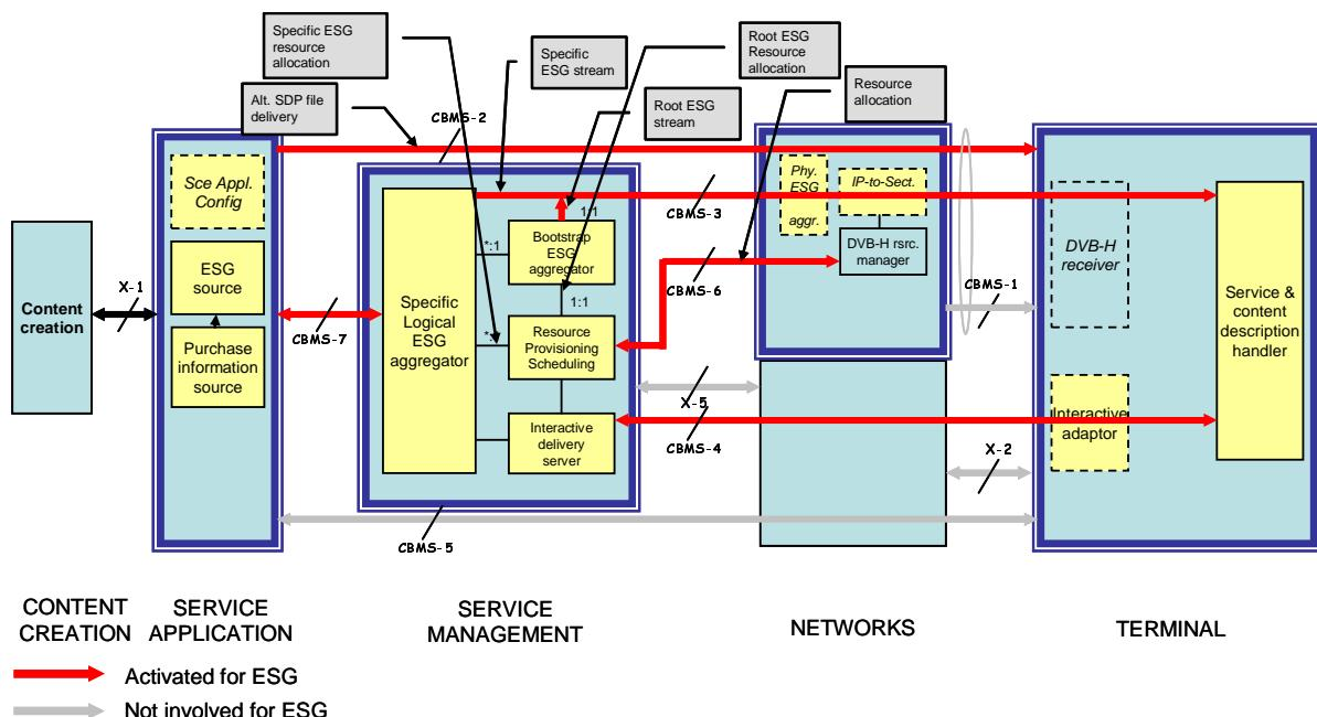
Figure 4: Reference points activated for ESG
