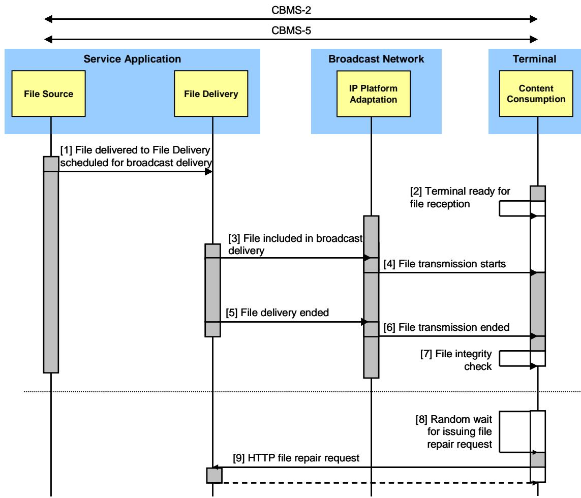
**Figure 12: Message flow for File Delivery**
