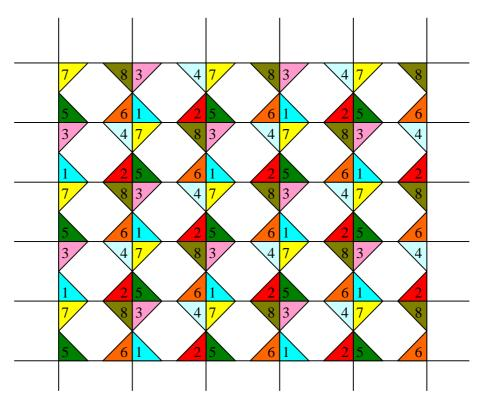
Figure B.6: Example 1 of frequency distribution, reuse factor = 2
