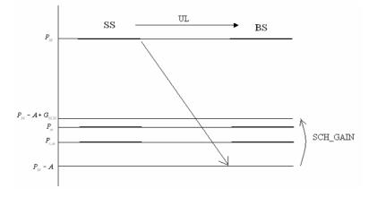
Figure B.5: ST transmits with maximum power level, but the received power level at BS is below the threshold
