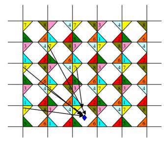
A Subscriber Station at the cell edge will see interference from the neighbour cells, as shown in figure B.9.
