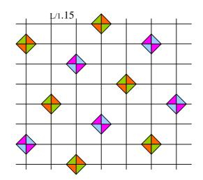
Figure B.7: Example 2 of frequency distribution, reuse factor = 2
