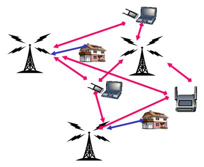
Figure C.1: Up-link interference in a converged Fixed-Nomadic system
