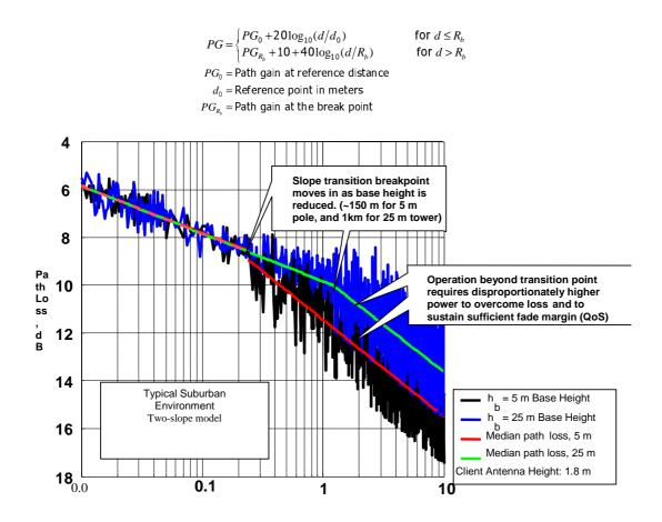
Figure B.10: Measured path loss at 2.4 GHz
