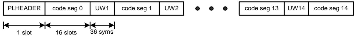
**Figure B.3: Pilot structure for 8PSK modulation, where UWs (unique words) refer to pilot symbols**
