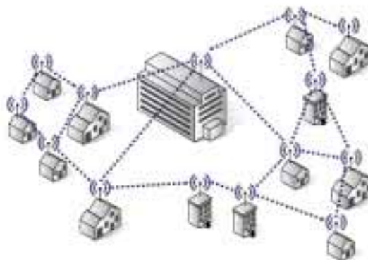
Figure 1: Mesh network example (any of the nodes may act as the access point)
