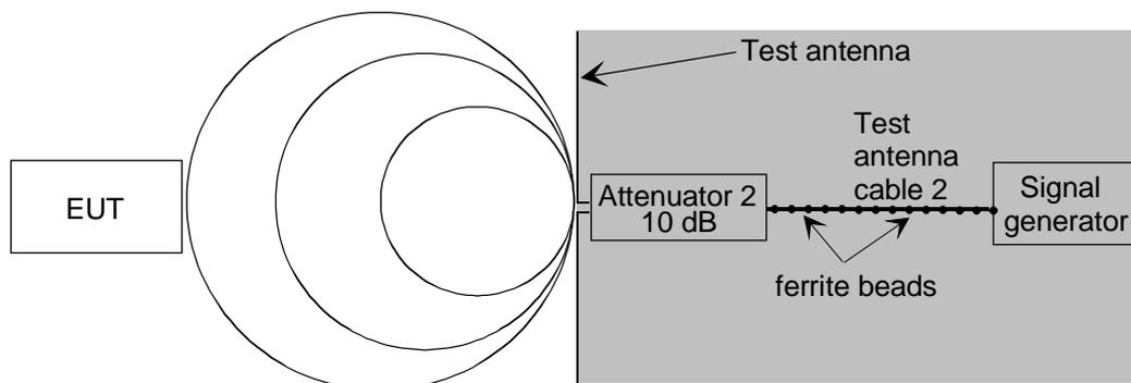
Figure 11: Stage 2: EUT measurement
