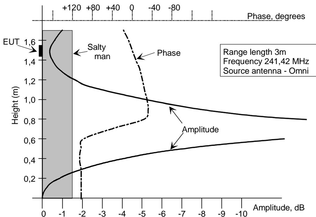
**Figure 5: Amplitude and phase distribution along the Salty man over a reflective ground**
