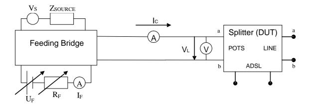
Figure 22: Test set-up for ringing impedance testing on a splitter at POTS Port
