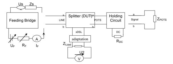
Figure 26: Test set up for noise testing in the ADSL band on a splitter at the xDSL port
