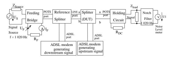
Figure 11: Test set-up for distortion testing on a splitter with ADSL signal
