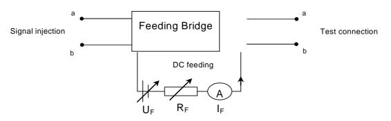
Figure 1: External circuitry for feeding bridge
