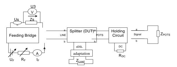
Figure 27: Test set up for noise testing in the ADSL band on a splitter at the xDSL port
