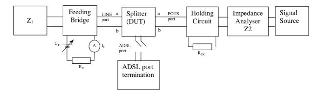
Figure 7: Test set-up for insertion loss testing on a splitter ( at the POTS Port )
