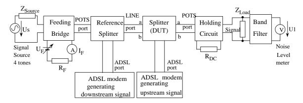
Figure 13: Test set-up for intermodulation testing on a splitter with ADSLsignal
