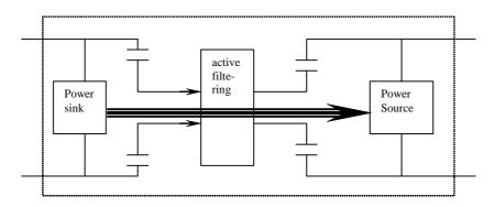
Figure 4: Example for a splitter breaking the DC path
