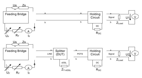
Figure 9: Test set-up for isolation testing on a splitter
