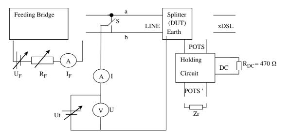
Figure 14: Test set-up for DC resistance between terminal and earth when testing LINE port
