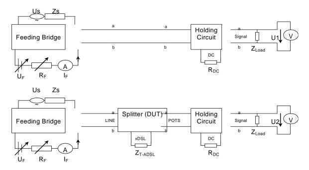
Figure 24: Test set-up for POTS band noise testing on a splitter
