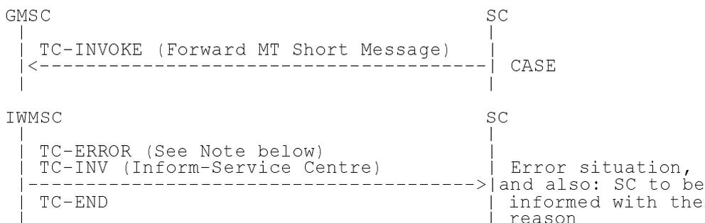
**NOTE:** The Inform-SC invoke component is always grouped with an error component of Forward Mobile Terminated Short Message operation, when sent to an SC. Which error component, is described in the Mapping of Errors chapters for the Forward Mobile Terminated Short Message operation.
