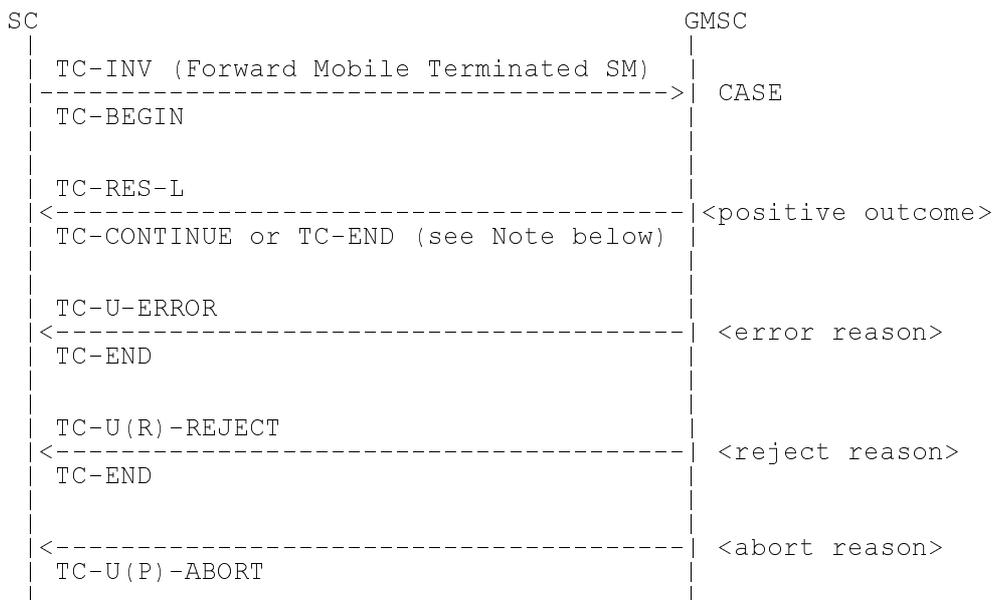
**NOTE:** If the 'moreMessagesToSend' flag is set to TRUE in the Forward Mobile Terminated SM invoke component, theResult component shall be sent in a Continue message. If it is set to FALSE, in an End message.
