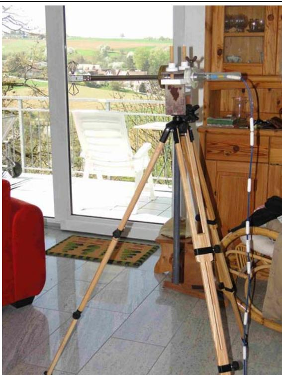
Biconical Antenna on wooden tripod
