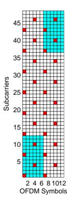
Figure A.6: Distributed VRB multiplexing in LTE DL
