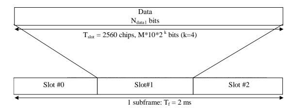
Figure 3: HSDPA Frame Structure [i.6]
