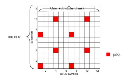
Figure 6: LTE downlink subframe TTI (2 RBs, extended CP); 1 ms duration
