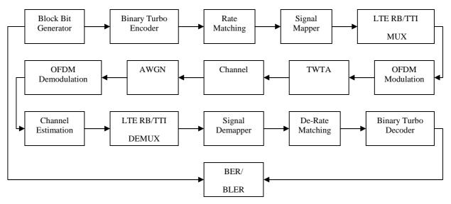
Figure A.3: Block diagram of the LTE link-level simulator
