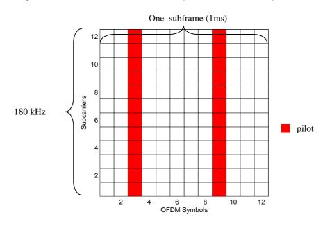
Figure 7: LTE uplink subframe TTI (2 RBs, extended CP); 1 ms duration
