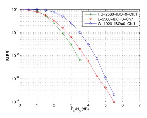
Figure B.8: Uplink performance comparison, saturated TWTA (long TTI)
