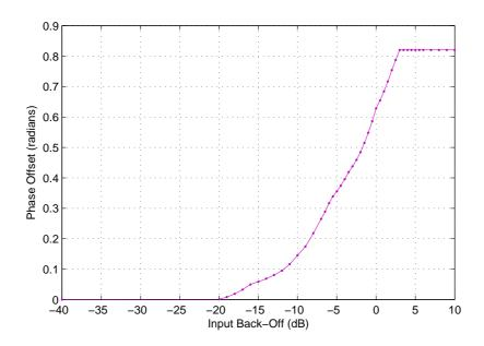
Figure 13: TWTA amplitude-to-phase response
