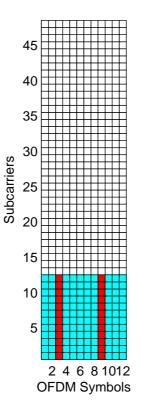
Figure A.5: Localized VRB multiplexing in LTE UL
