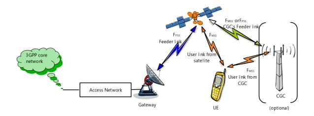
Figure 2: Mobile satellite system architecture
