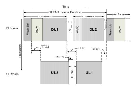
Figure 9: WiMAX frame structure example (FDD)
