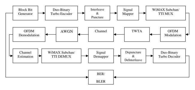
Figure A.4: Block diagram of the WiMAX link-level simulator
