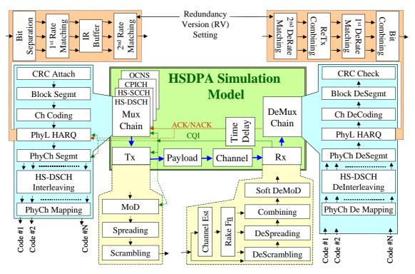
Figure A.1: HSDPA Simulation Model
