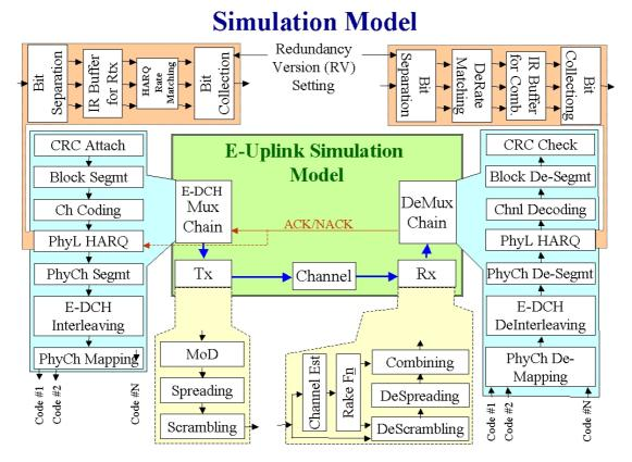
Figure A.2: HSUPA Simulation Model
