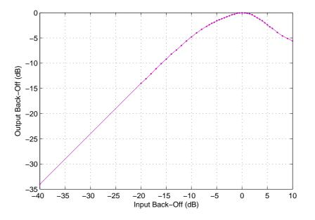
Figure 12: TWTA amplitude-to-amplitude response
