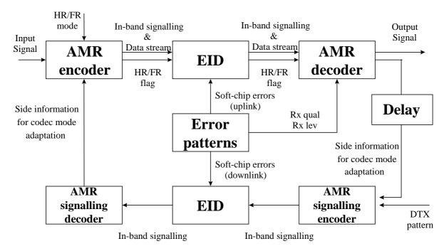
Figure 9.1: Block diagram of the AMR speech traffic channel simulation model
