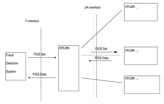
Figure 1: Flow of messages between the HPLMN and the VPLMN and between the HPLMN and the FDS
