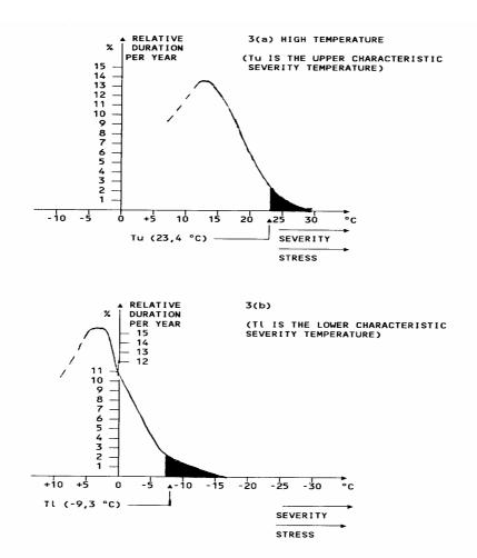
Figure 3: Separated distributions of outdoor air temperature showing the boundary value of the upper (Tu) and the lower (TI) characteristic temperature
