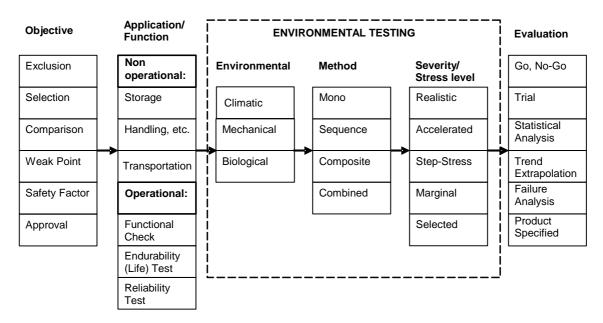
Figure 5: Outline of environmental testing applications
